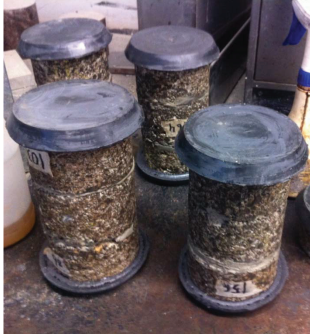
Figure 3-18 Dynamic modulus sample glued and capped
