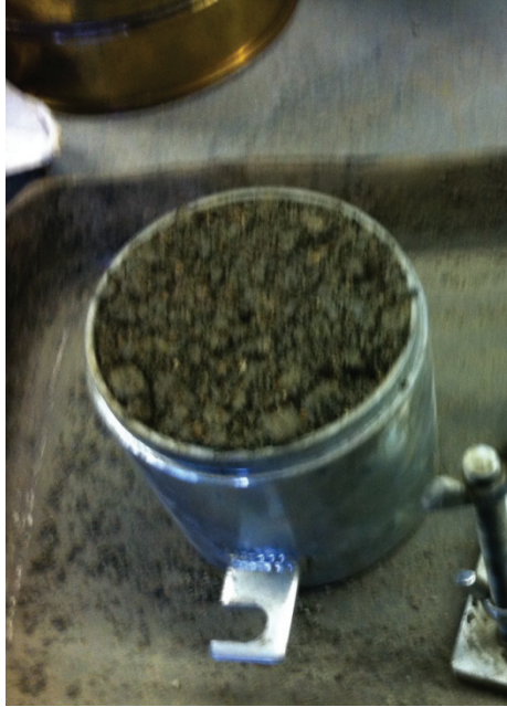
Figure 3-2 Compacted sample in Proctor mould
