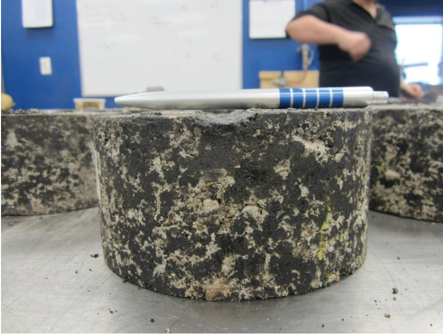
Figure B-43 Mix 4, Sample 1 rutted sample
