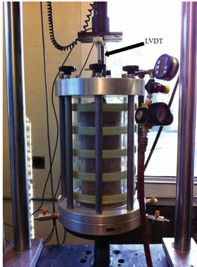
Figure 3-5 Triaxial chamber setup on load frame
