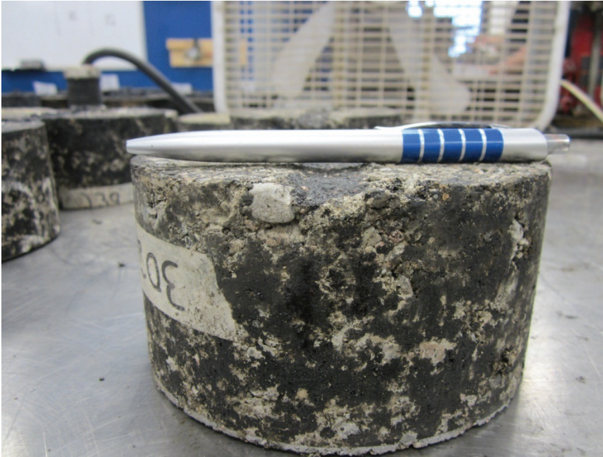
Figure B-33 Mix 2, Sample 1 rutted sample
