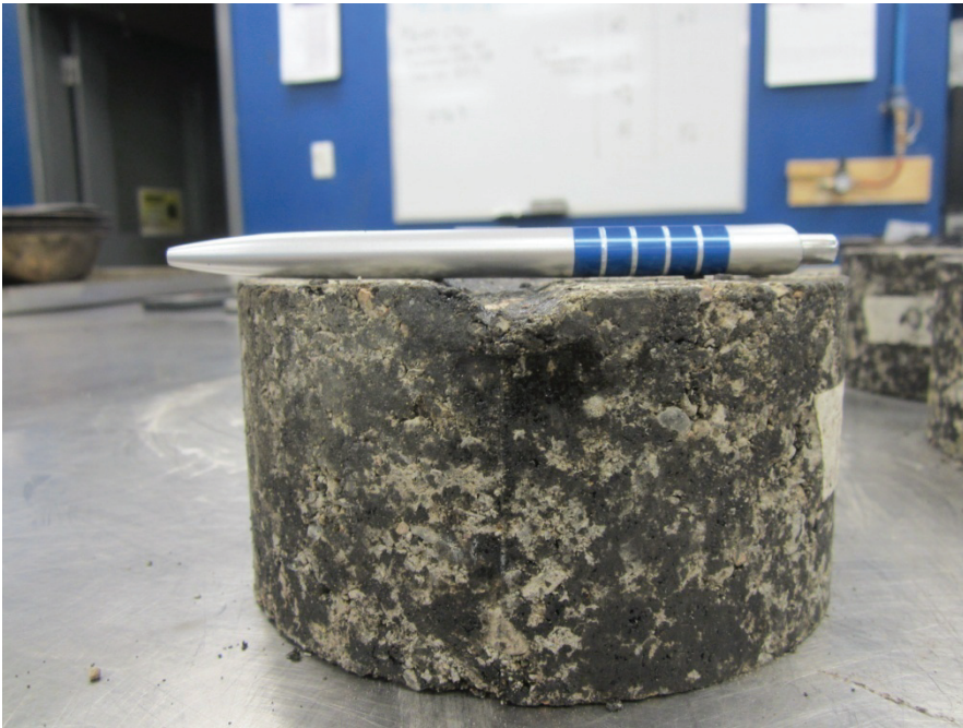
Figure B-59 Mix 7, Sample 2 rutted sample
