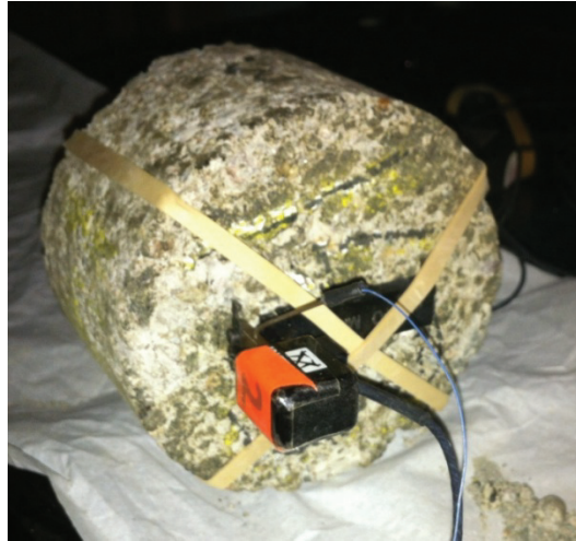
Figure 3-17 Dynamic extensometer mounted on resilient modulus sample
