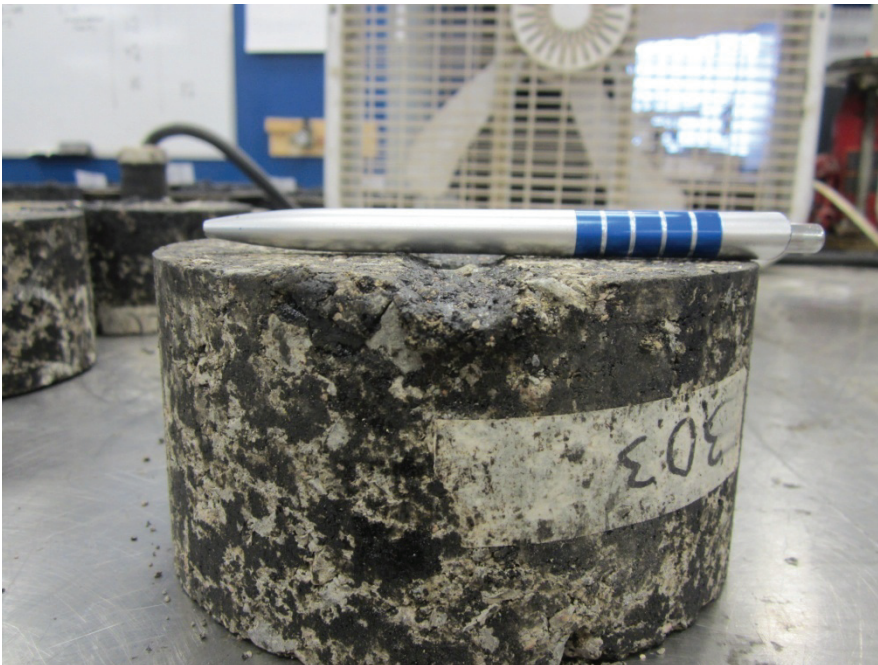
Figure B-34 Mix 2, Sample 2 rutted sample
