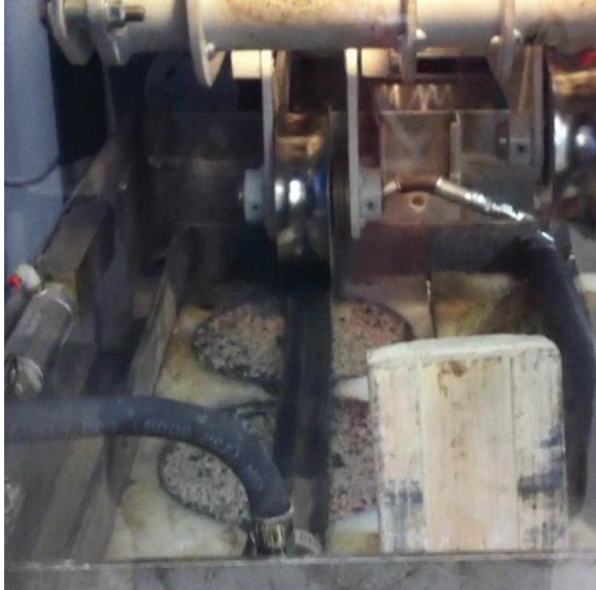
Figure 3-20 Two samples for rutting test in the Asphalt Pavement Analyzer
