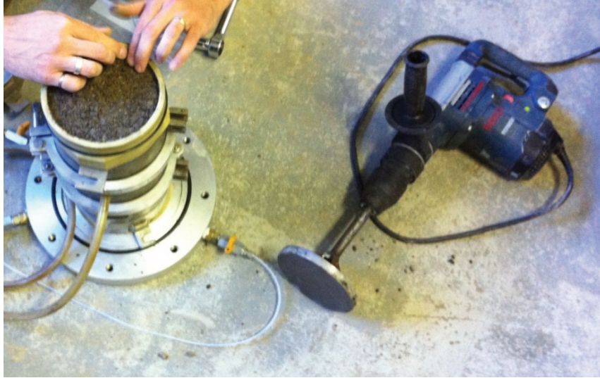
Figure 3-3 Vibratory compaction of resilient modulus sample
