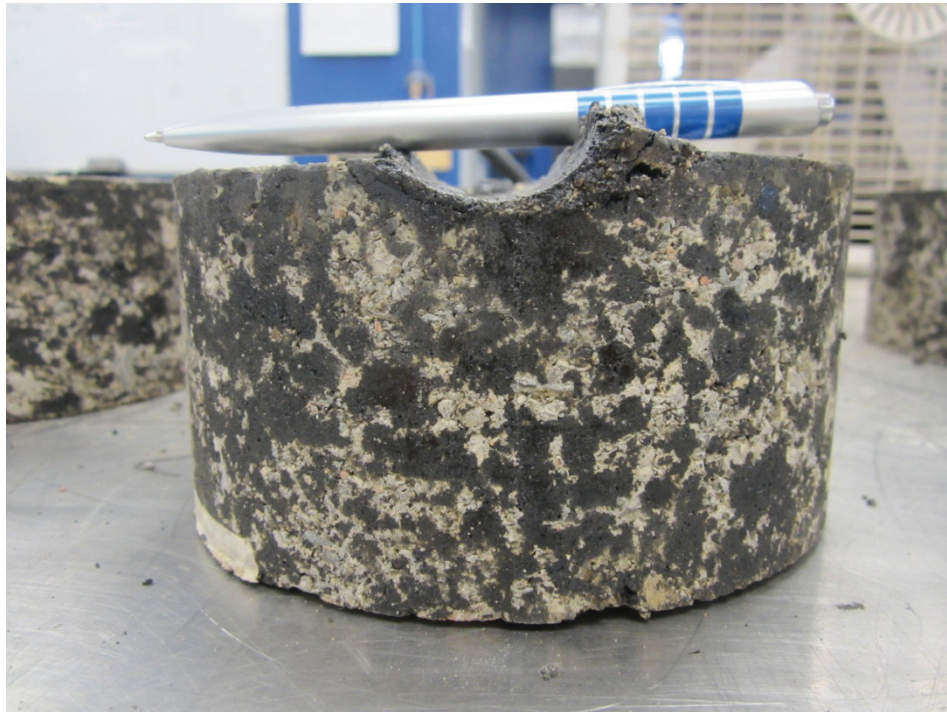
Figure 2-15 Sample after rutting test
