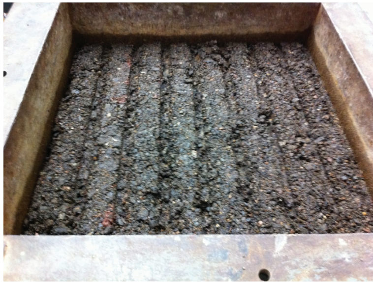
Figure 3-6 Compacted direct shear test sample
