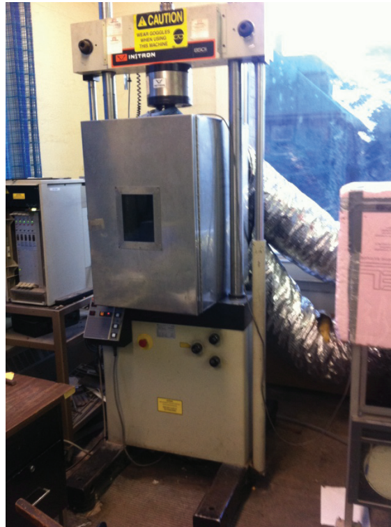
Figure 2-13 Dynamic modulus testing machine and environmental chamber
