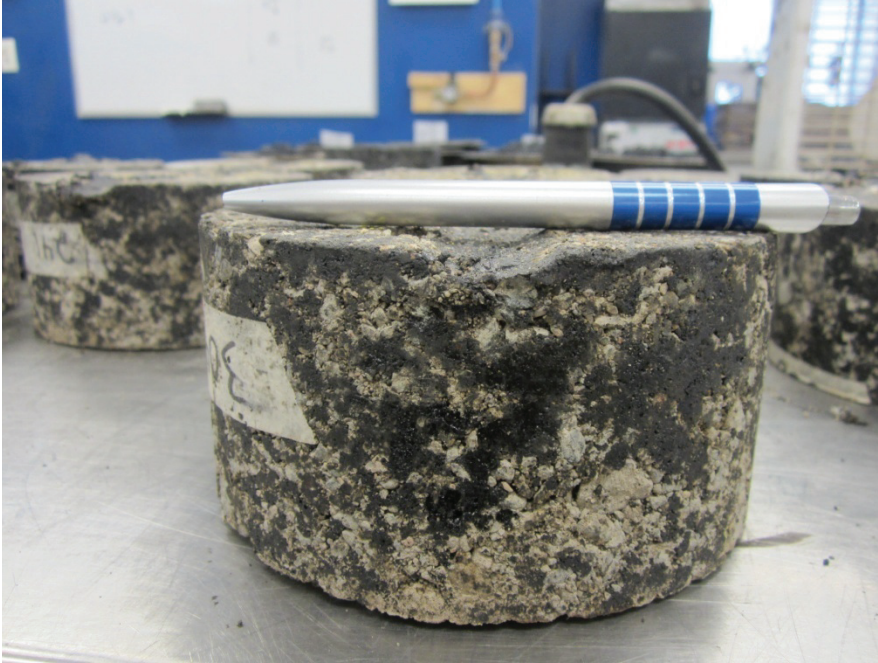
Figure B-28 Mix 1, Sample 1 rutted sample
