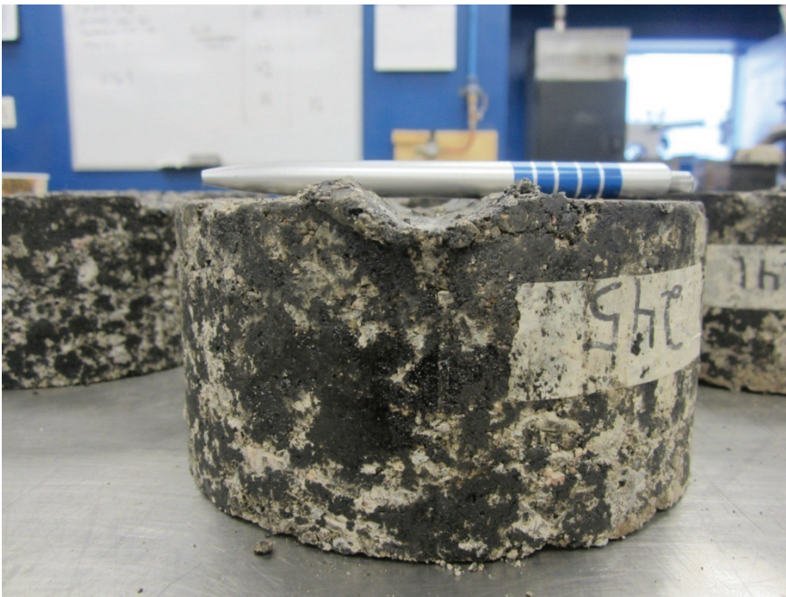
Figure B-39 Mix 3, Sample 2 rutted sample
