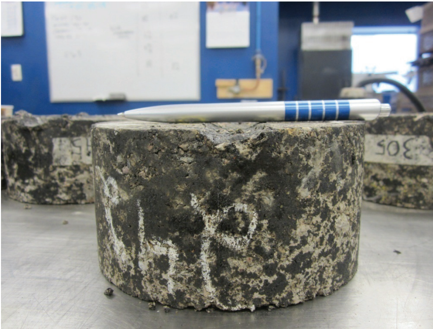
Figure B-49 Mix 5, Sample 2 rutted sample
