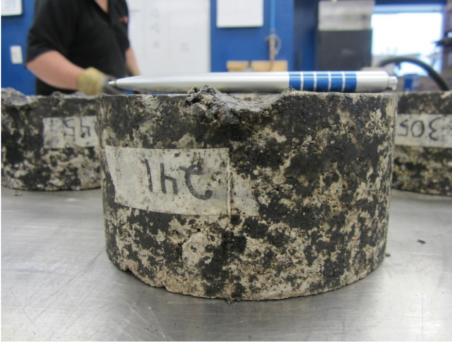
Figure B-48 Mix 5, Sample 1 rutted sample
