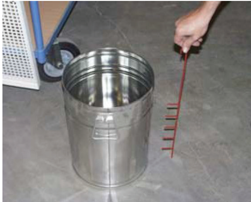
Figure 3-9 Bucket and dipstick for evaluating asphalt foaming characteristics (Wirtgen Group, 2010)
