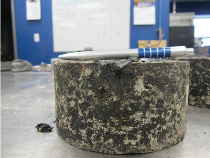
Figure B-58 Mix 7, Sample 1 rutted sample
