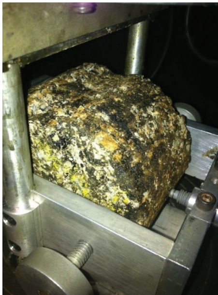
Figure 3-16 Resilient modulus sample setup using LVDTs to record deformation
