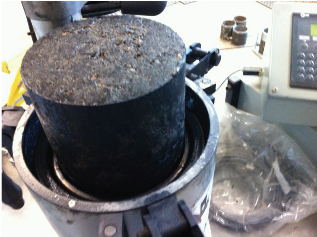
Figure 3-14 Gyratory sized sample
