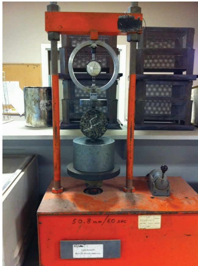
Figure 3-15 ITS testing apparatus
