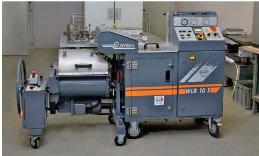
Figure 2-18 Wirtgen WLB-10S laboratory plant and WLM-30 pugmill mixer (Wirtgen Group, 2010)
