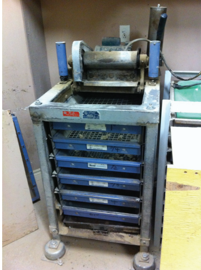
Figure 3-8 Gilson Company Inc. testing screens used to split material by size
