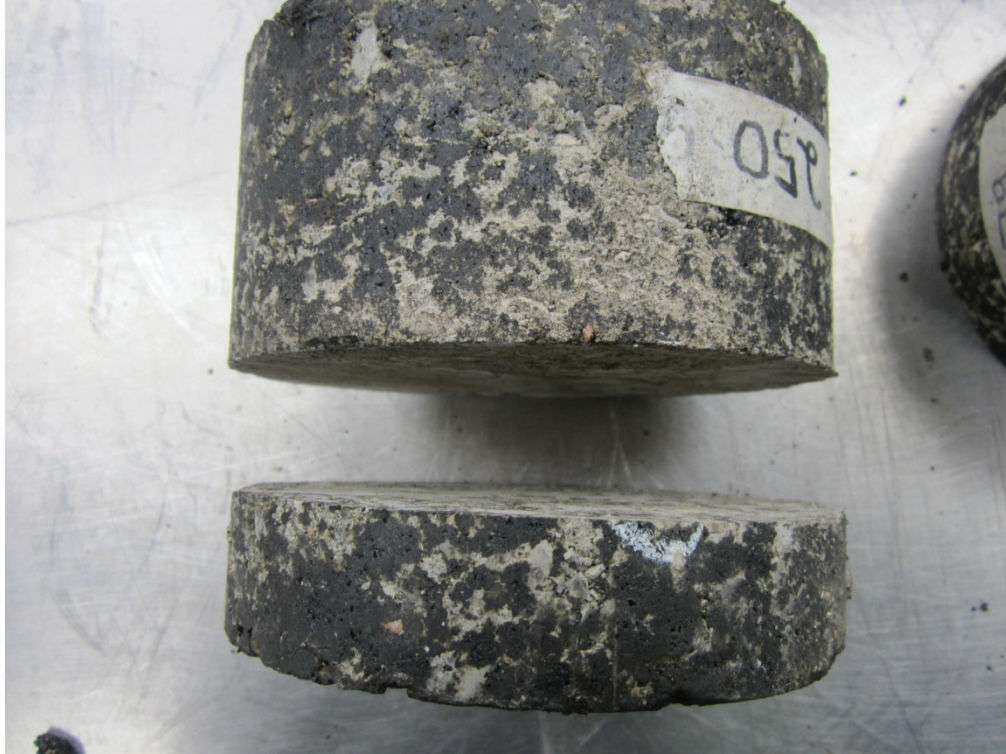
Figure 3-19 Gyratory sized sample after cutting for rutting testing.
