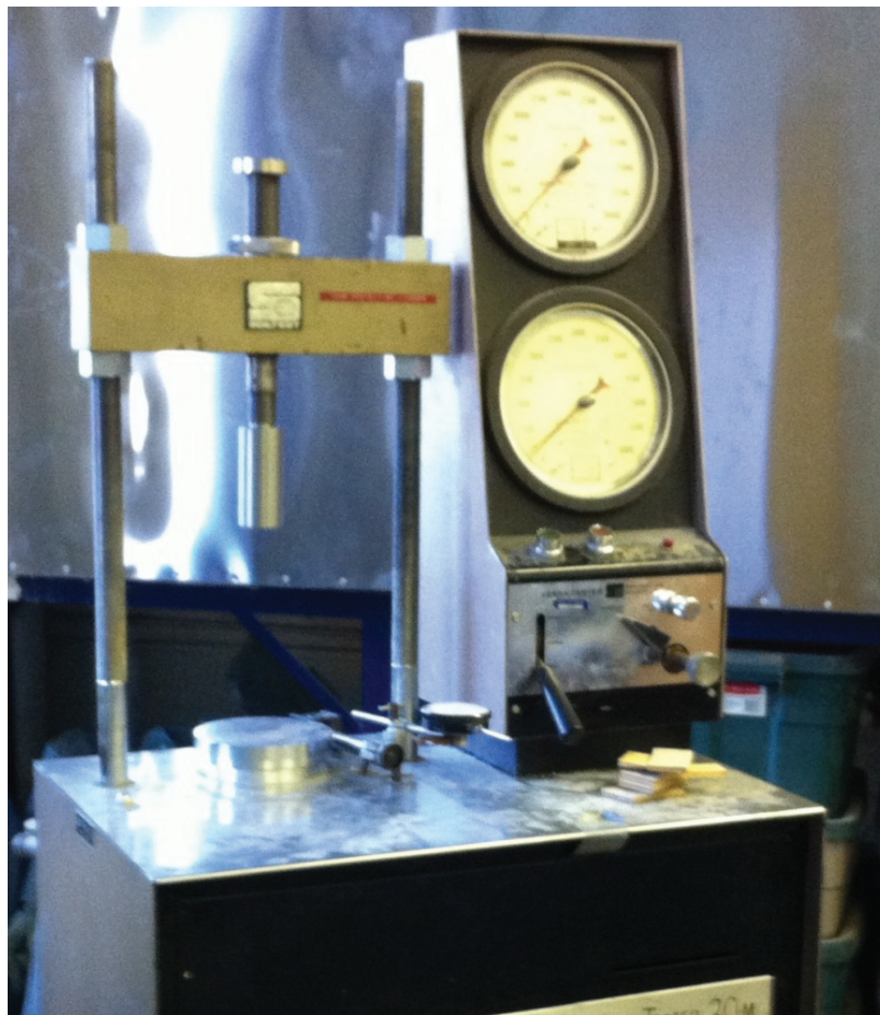
Figure 3-7 CBR testing machine
