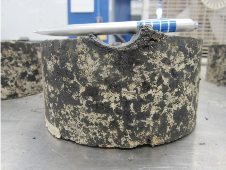
Figure B-53 Mix 6, Sample 1 rutted sample
