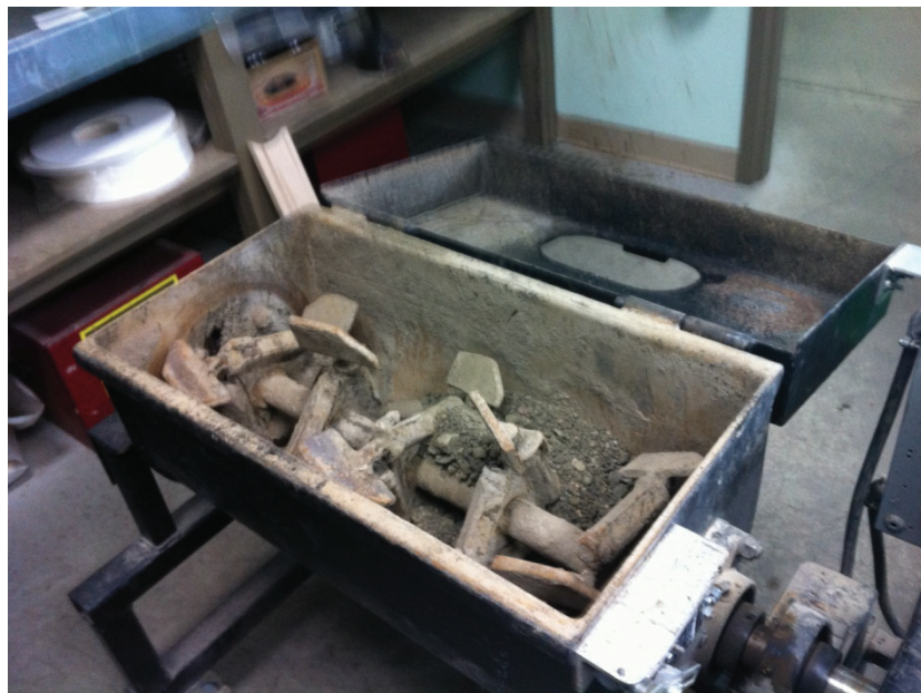
Figure 3-11 Wirtgen laboratory scale pugmill mixer
