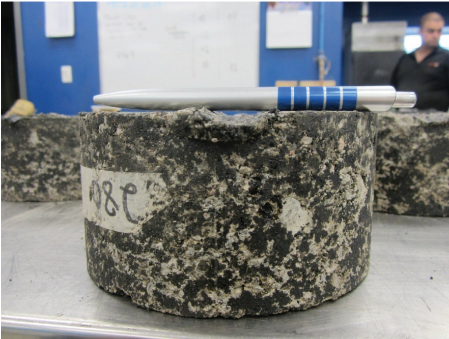
Figure B-44 Mix 4, Sample 2 rutted sample
