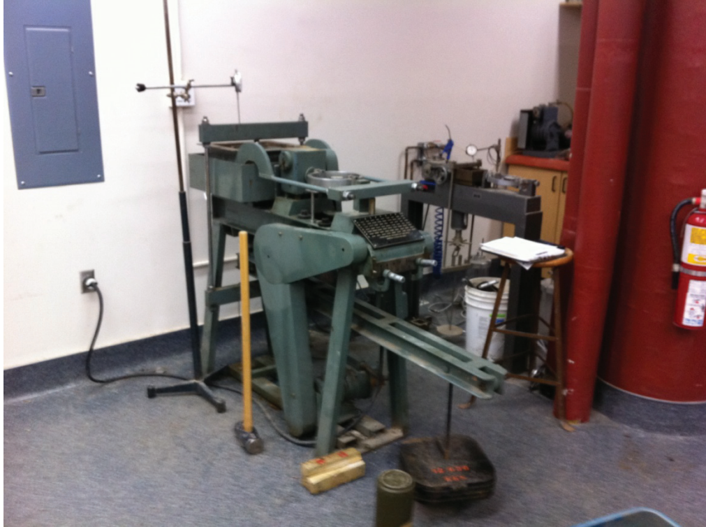
Figure 2-6 Direct shear testing apparatus
