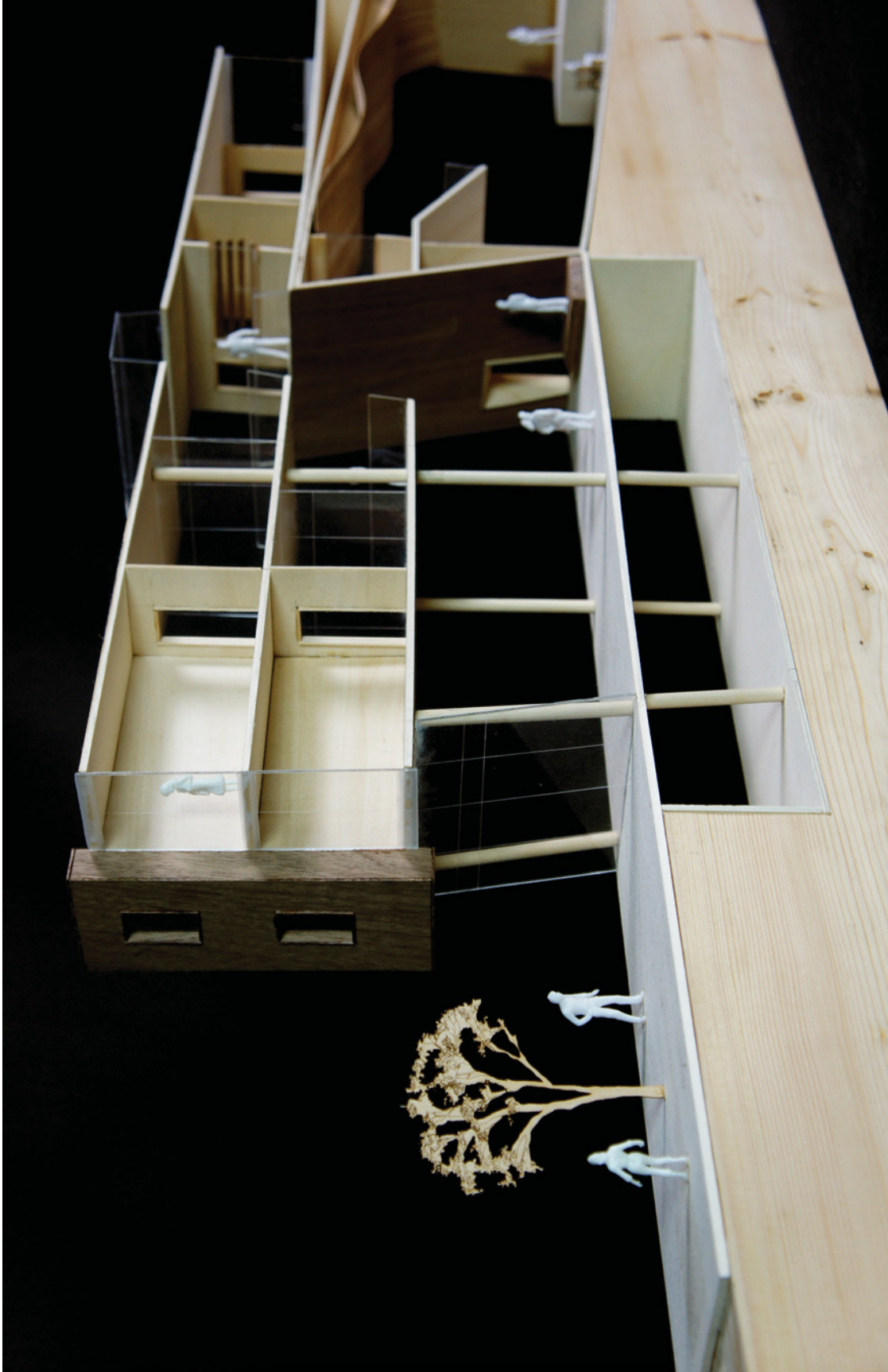
Detail of long section model showing building entry, office spaces and atrium with casual performance space.
