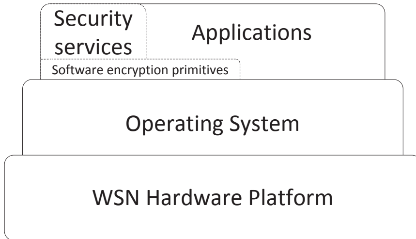
Figure 5.1 Wireless node design using software cryptography over unsecure platform
