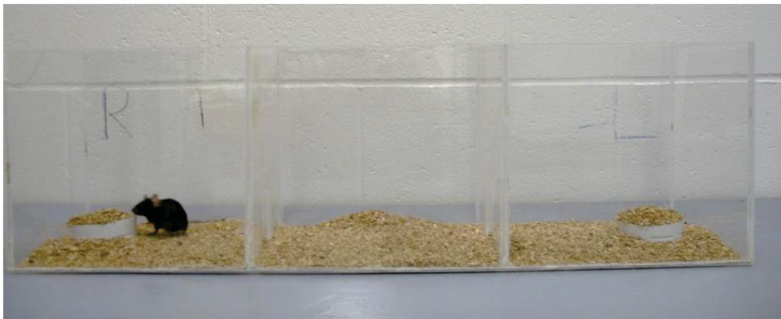
Figure 5.1. (A) The olfactory discrimination training apparatus consists of a housing cage filled with a bedding of pro-chip, and contained a single odor cup with either the CS+ or CS- odor. (B) The preference test apparatus consisted of a rectangular box made of transparent plexiglas, and was divided into three chambers of equal size. Walls between adjacent chambers each contained a small door, and the test apparatus contained a bedding of pro-chip. CS+ and CS- odor pots without sugar reward were placed in chambers at opposite ends of the apparatus.
