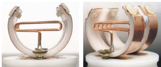
FIG. 3. (Color online) Photographs of a rotatable flat coil holder built for a Chemmagnetics Apex DRNS Wideline static solid-state NMR probe.
