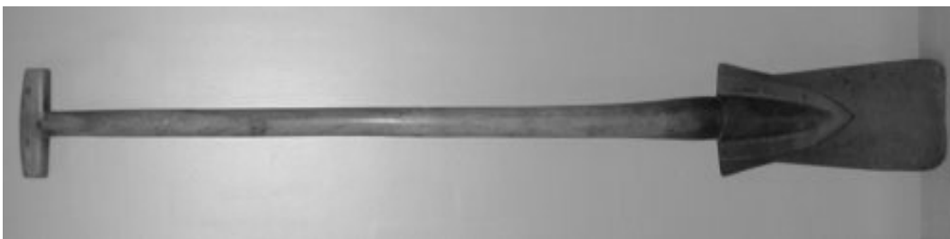
Figure 2.2: A type of dyking spade used by Acadians in building dykes. It was a simple yet effective tool. This dyking spade was made by Charles A.D. Siddall (length 104 cm) (Source: MacKinnon, 2004).
