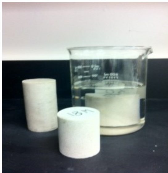
Figure 3.1 Fontainebleau sandstone core
