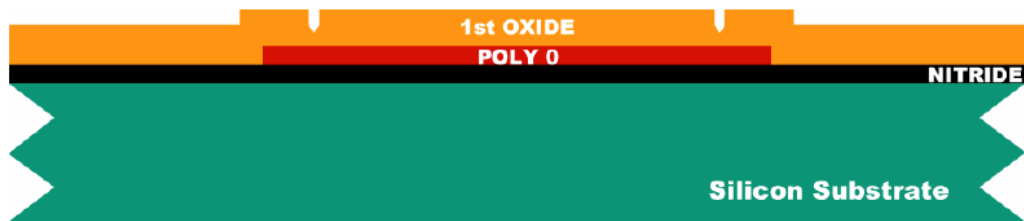
FIGURE 1.6. The wafers are coated with photoresist and the second level (DIMPLE) is lithographically patterned. The dimples, 750 nm deep, are reactive ion etched (RIE) into the first oxide layer. After the etch, the photoresist is stripped.
