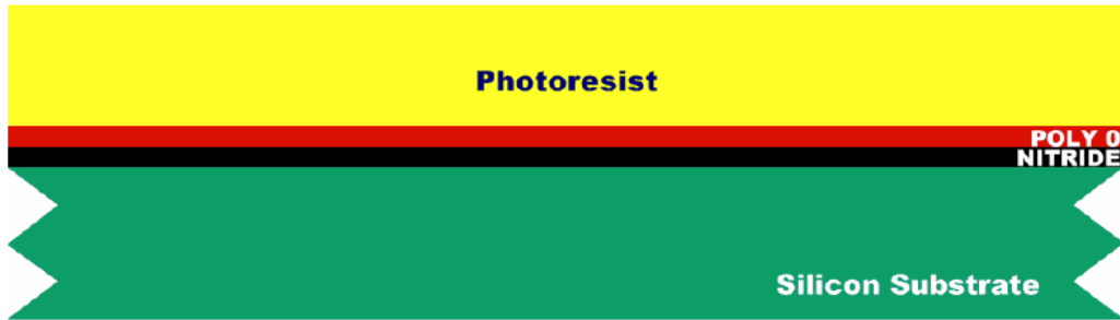
FIGURE 1.2. The surface of the starting n-type (100) wafers are heavily doped with phosphorus in a standard diffusion furnace using a PSG film as the dopant source. After removal of this PSG film, a 600 nm blanket layer of low stress silicon nitride (Nitride) is deposited followed by a blanket layer of 500 nm polysilicon (Poly 0). The wafers are then coated with UV-sensitive photoresist.
