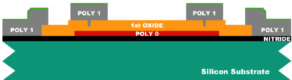
FIGURE 1.9. The wafer is coated with photoresist and the fourth level (POLY1) is lithographically patterned. The PSG is first etched to create a hard mask and then Poly 1 is etched by plasma processing. After the etch is completed, the photoresist and PSG hard mask are removed.
