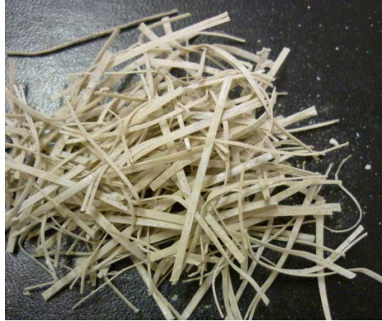
Figure 5.30 - Washout sample of fiber containing HDPE and 10% EVA
