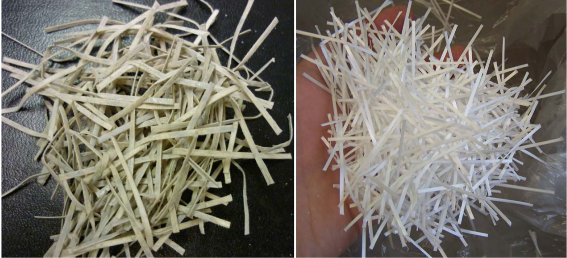
Figure C-155 - Washout sample and virgin sample of cut prototype fiber containing HDPE, 11% PVDF and 20% MAH
