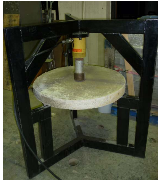
Figure 4.28 - Test setup for ASTM C1550-10
