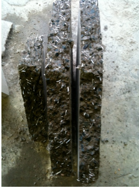
Figure 4.29 - Fully broken round panel specimen
