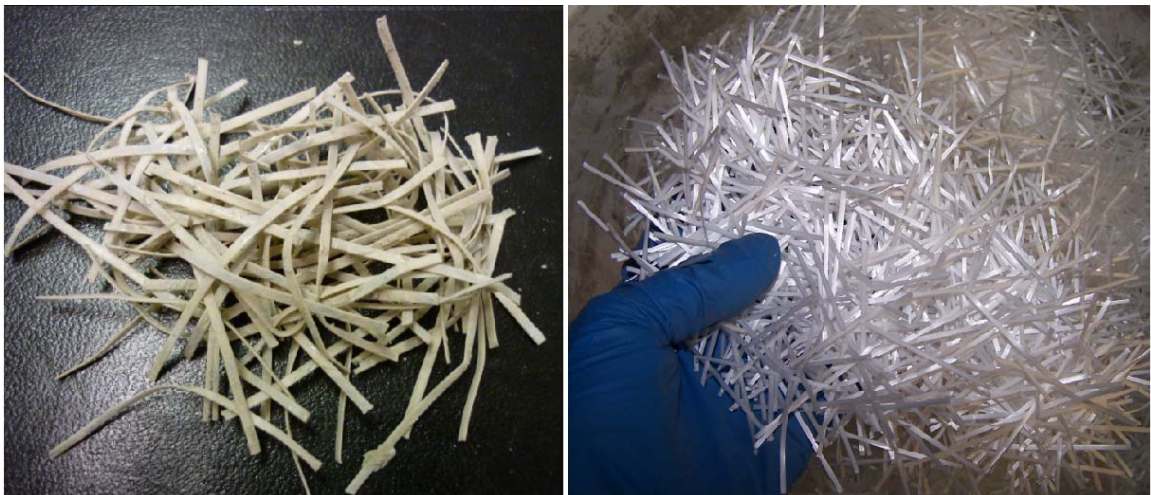
Figure C-150 - Washout sample and virgin sample of cut prototype fiber containing HDPE and 1% PVDF
