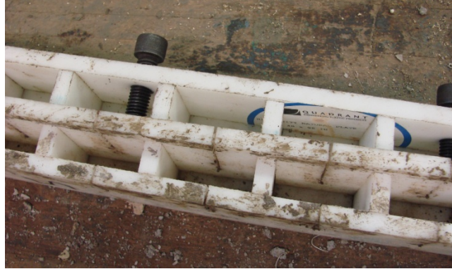
Figure 4.7 - Mold used for pullout specimen
