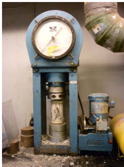
Figure 2.23 - Cylinder failed in compression in testing machine
