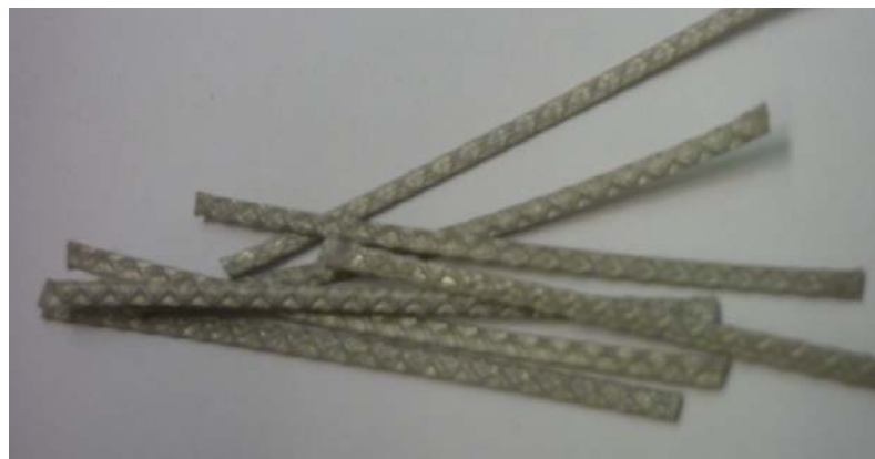
Figure 3.21 - Embossed pattern on “Bar Chip” brand polyolefin fiber
