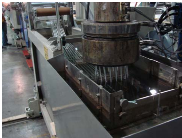
Figure 2.7 - Filament extrusion using melt spinning
