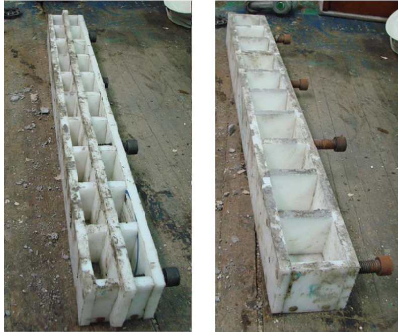
Figure 4.6 - Molds for pullout specimens and mortar cubes
