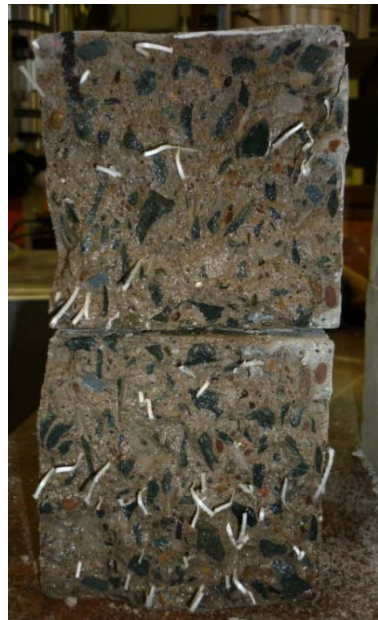
Figure 5.32 - Break face of outlier sample from ASTM C1399 testing for fiber containing HDPE, 7% PVDF and 10% MAH
