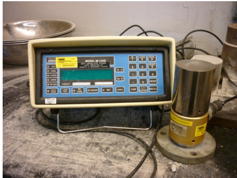
Figure 4.19 - Load cell and readout used for compression testing of mortar cubes
