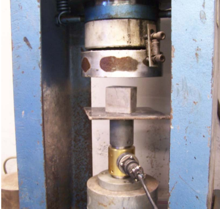
Figure 4.18 - Test setup for compression of mortar cube
