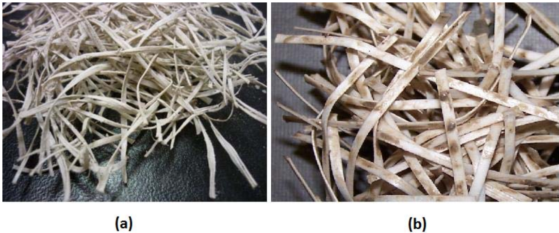
Figure 5.29 - Washout samples of prototype fibers containing (a) PP, 10% HDPE and 10% EVA, illustrating fibrillation and (b) HDPE and 3% PVDF, illustrating no fibrillation
