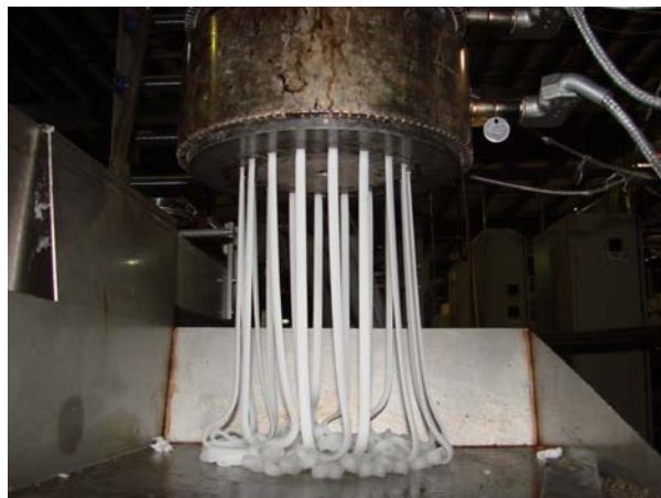
Figure 2.5 - Spinneret extruding polyolefin material
