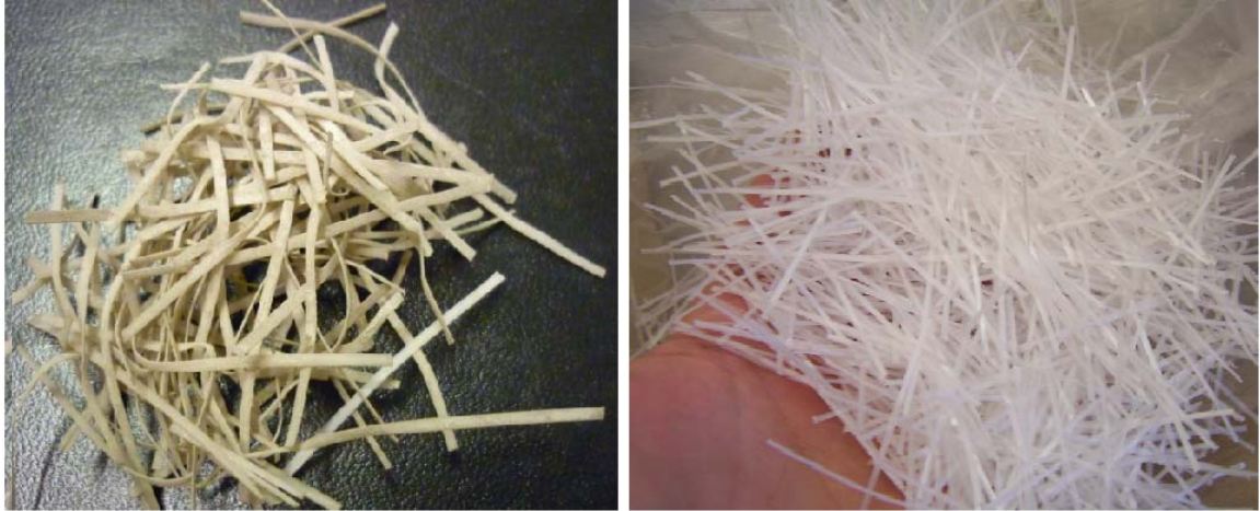
Figure C-149 - Washout sample and virgin sample of prototype fiber containing 100% HDPE
