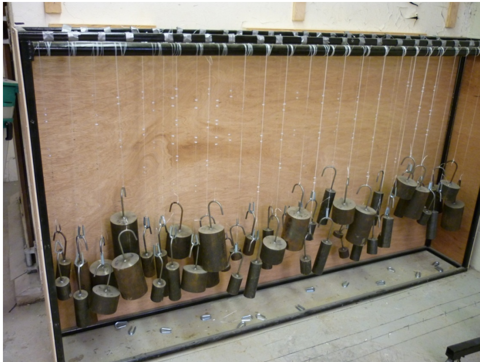
Figure 4.30 - Test setup for fiber tensile creep testing
