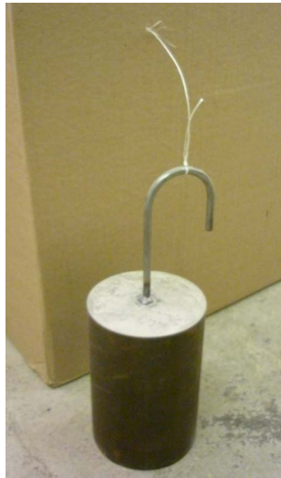
Figure 5.45 - Ruptured filament and weight
