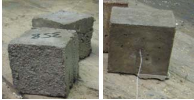
Figure 4.9 - Mortar cubes and pullout specimens after demolding, before moist curing
