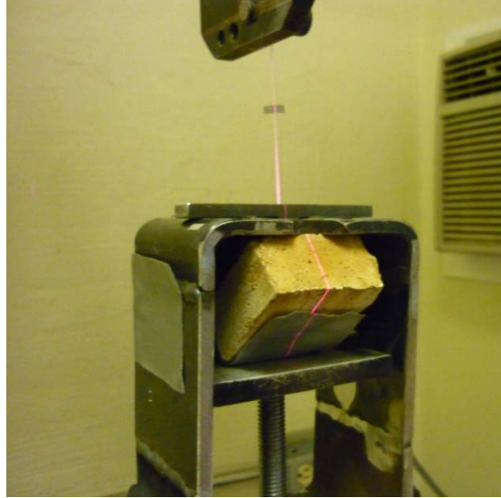
Figure 4.17 - Pullout specimen undergoing inclined pullout
