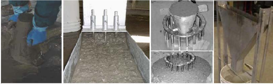
Figure 3.18 - Testing methods for SCC. From left: Slump flow, L-box, J-Ring and V-funnel tests (Forgeron & Omer, 2010), (ASTM International, 2009)
