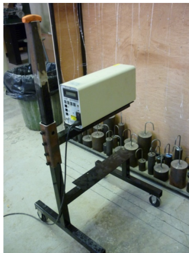
Figure 4.32 - Laser extensometer on adjustable dolly
