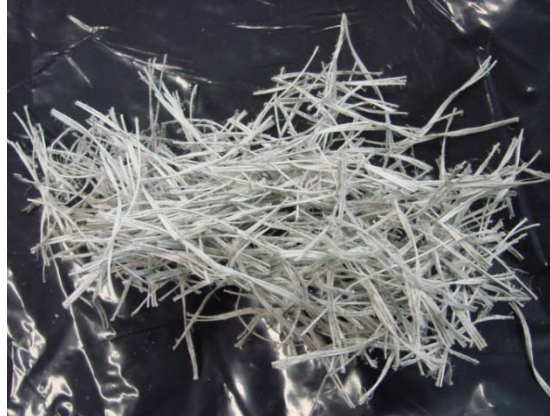
Figure 4.22 - A washout sample showing visible fibrillation
