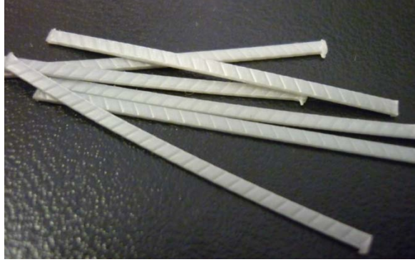
Figure 4.20 - BASF MasterFiber MAC470 embossed fibers
