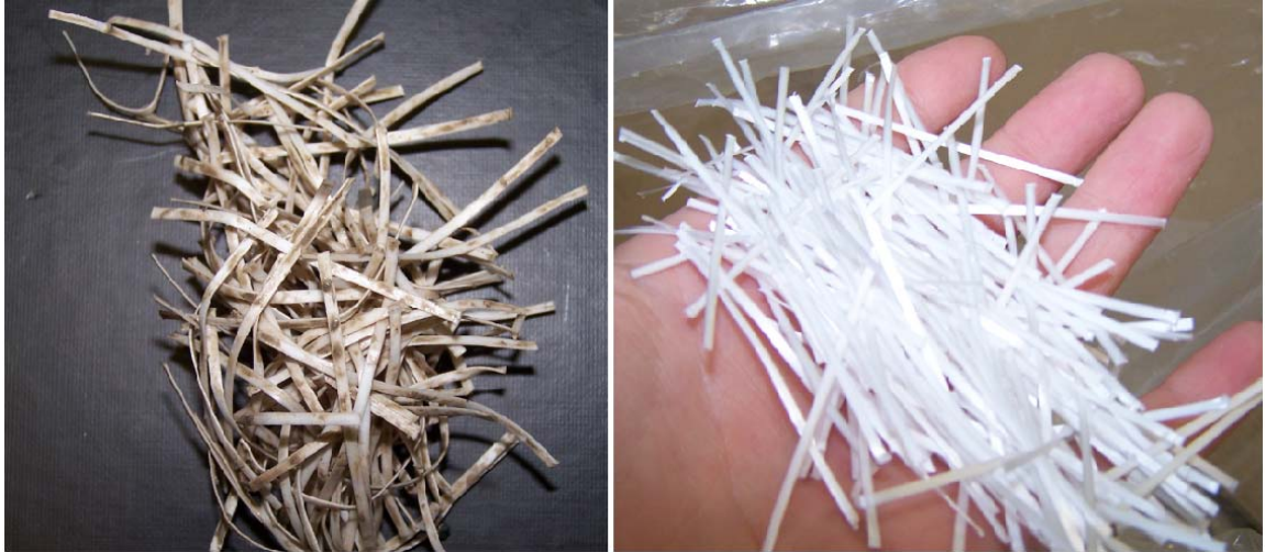
Figure C-151 - Washout sample and virgin sample of cut prototype fiber containing HDPE and 3% PVDF
