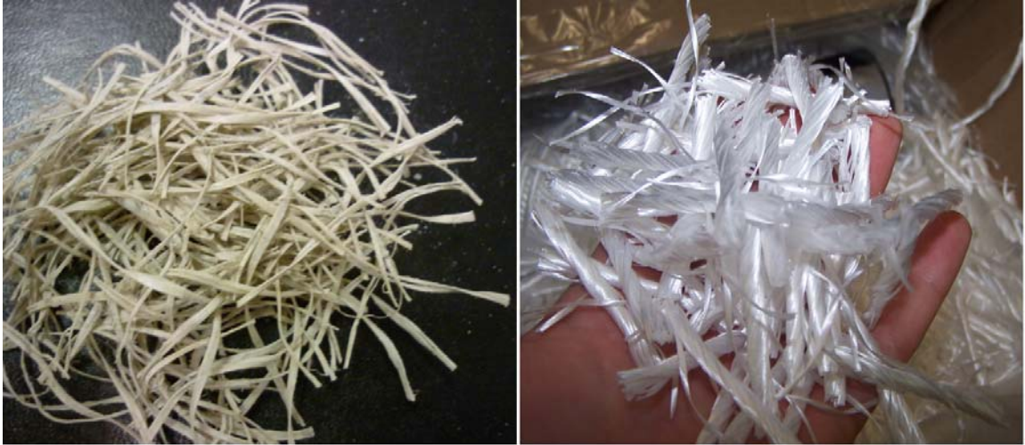
Figure C-157 - Washout sample and virgin sample of cut and twisted prototype fiber containing PP, 10% HDPE and 10% EVA
