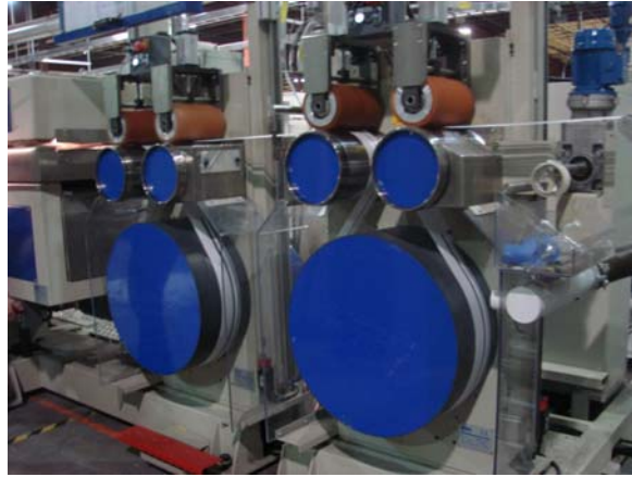
Figure 2.8 - Godets used to stretch filaments on an extrusion line
