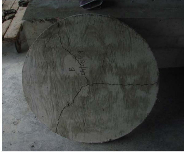
Figure 2.29 - Typical fracture pattern of round panels after testing
