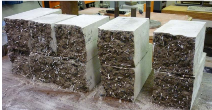
Figure 4.27 - Fully broken beam specimens
