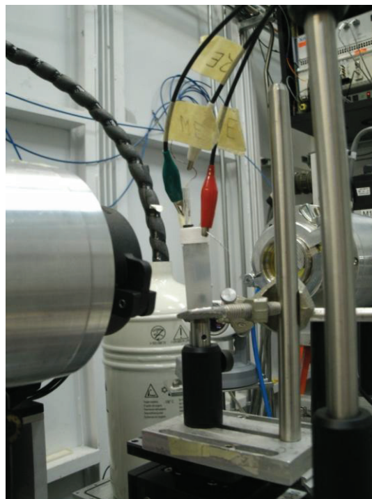
Figure 24: Alignment of the in situ electrochemical cell at the HXMA beamline (CLS).
