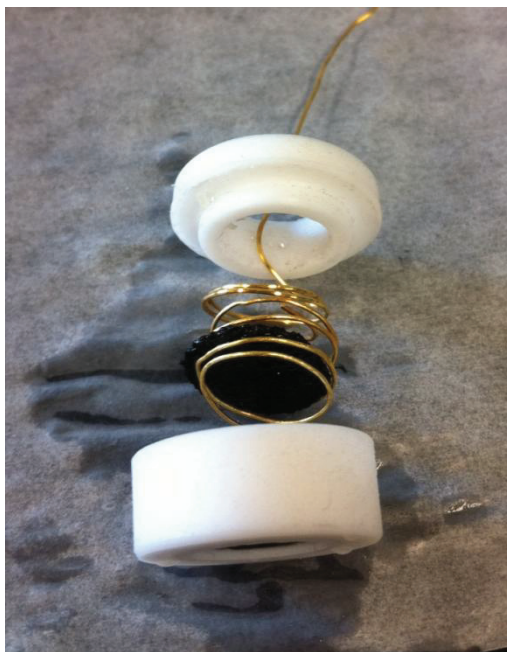
Figure 41: Custom carbon cloth electrode holder.
