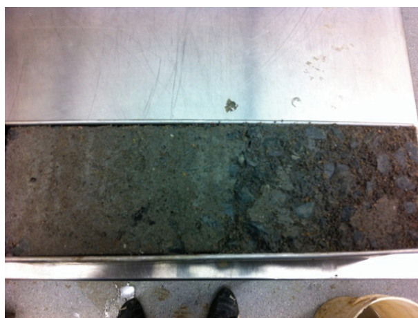
Figure 5.12 Broken FA Freeze Thaw Sample
