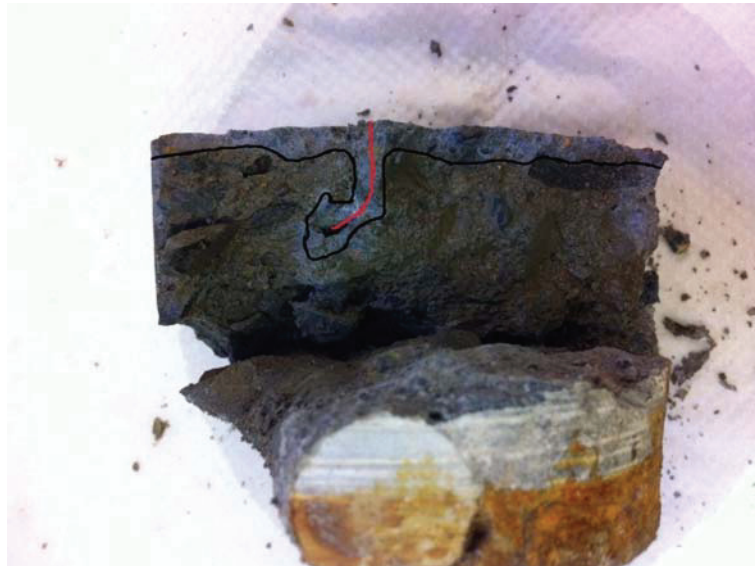
Figure 5.6 TER 50-1 Cracked Sample
