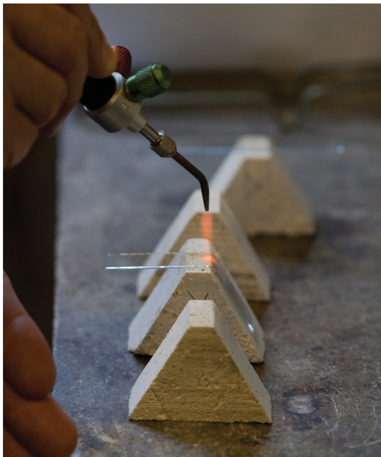
Figure 1.3: A photo of the glass being bent for the cuvette using a hydrogen-oxygen flame.
