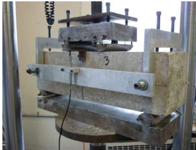
Figure 3.2 – Test set up for ASTM C1609-10
