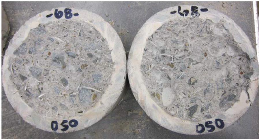
Figure 3.4 – Example of cylinder cross section with specimen number (bottom) and fibre count (top)
