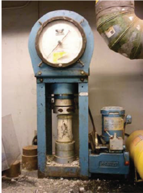
Figure 2.18 – Testing machine with sample failed in compression
