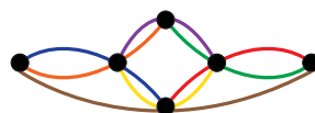
Figure B.1: The 3-uniform hypergraph on 6 vertices with 7 edges and uniformity dimension 3
