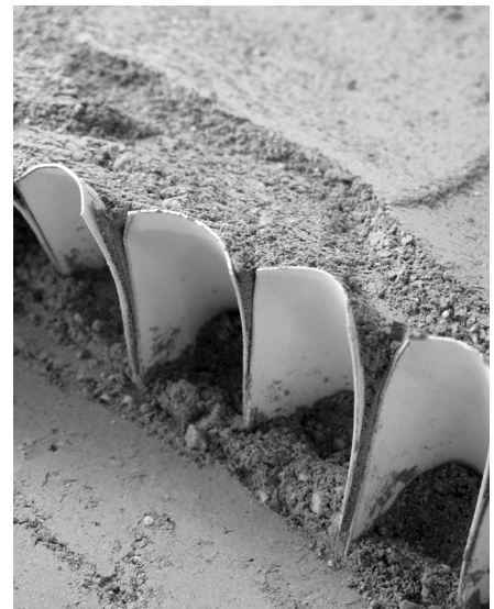
Sand model with scalloped forms creating habitable space and illustrating compressive forces.
