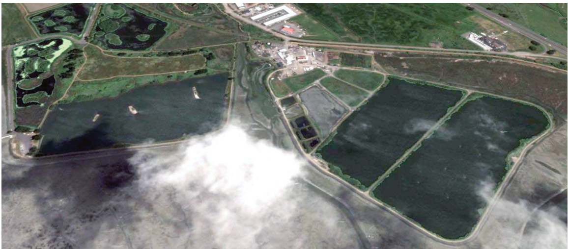
Aerial view of Arcata Marsh and Wildlife Sanctuary, California. The site features extensive wetlands used for treating municipal wastewater. (Google Earth 2012)
