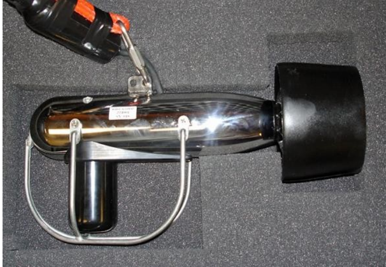
Figure 6.1: Towfish and 25 kHz transducer, WHOI photo [109]. The transducer is the black cylinder in the lower left of the photograph
