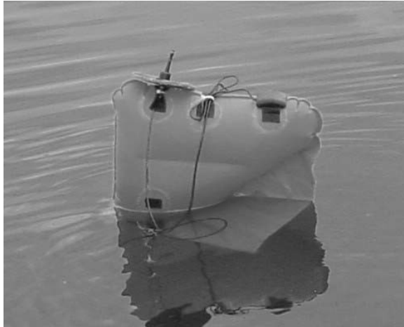
Figure 2.2: Float for the Florida Atlantic University air-droppable GATEWAY buoy, from [62]
