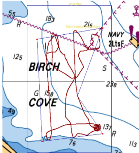
Figure 6.5: Reactive side scan sonar survey of non-convex polygon approximately 200 \times 300 m using [6]
