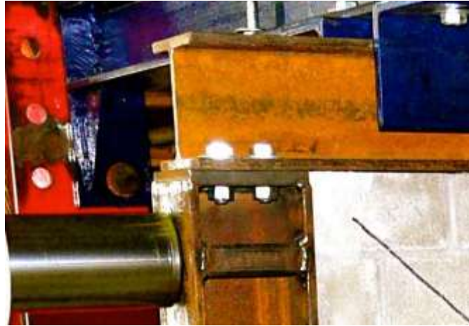
Figure 3.8 Initial Beam-to-column connection detail.
