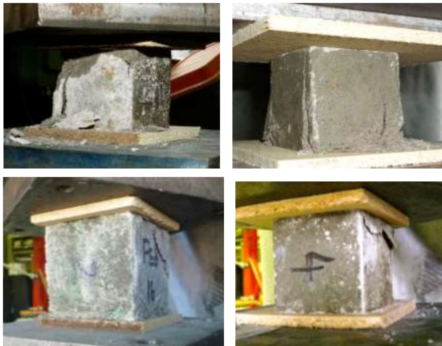
Figure 4.3 Failure of mortar cubes under compressive testing
