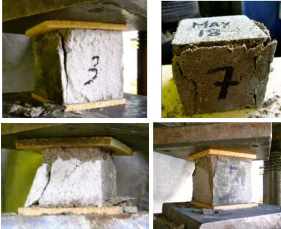
Figure 4.4 Failure of grout cubes under compressive testing
