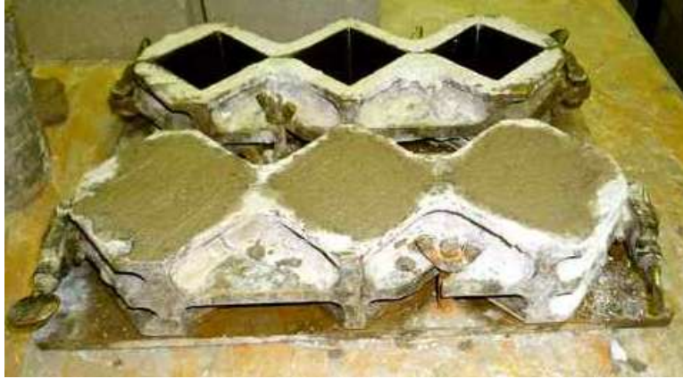
Figure 3.18 Mortar cubes in mold
