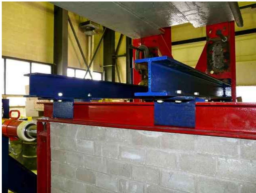
Figure 3.13 Out of plane support
