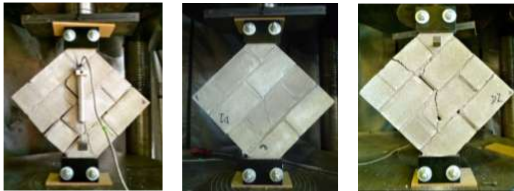
Figure 4.15 Diagonally loaded square prisms
