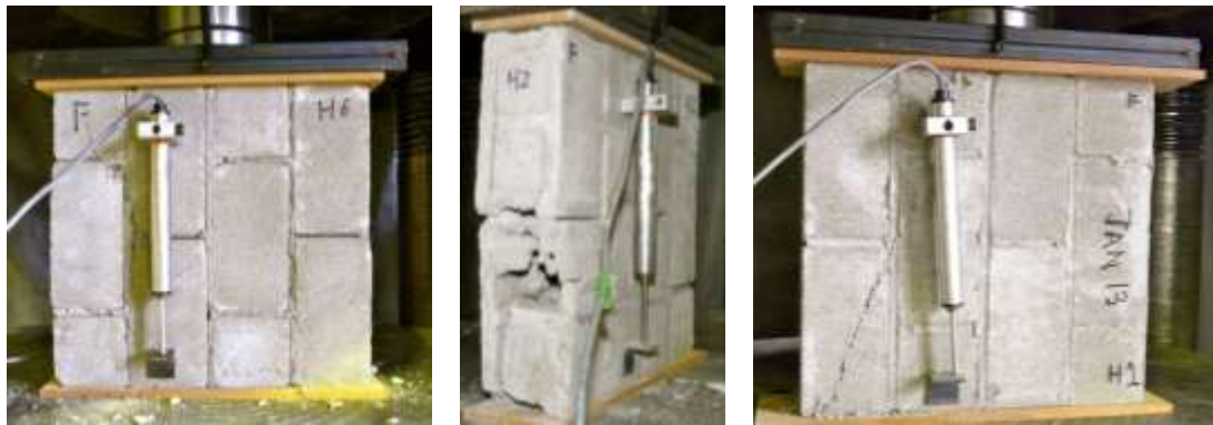
Figure 4.14 Horizontally loaded square prisms
