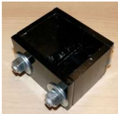
Figure 3.22 Diagonal prism test loading shoe.
