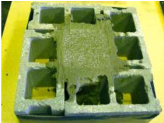
Figure 3.19 Grout cube molds
