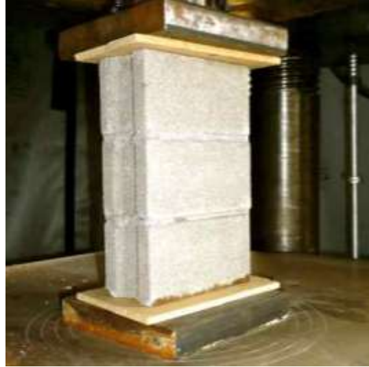
Figure 3.20 3-High Prisms testing arrangement
