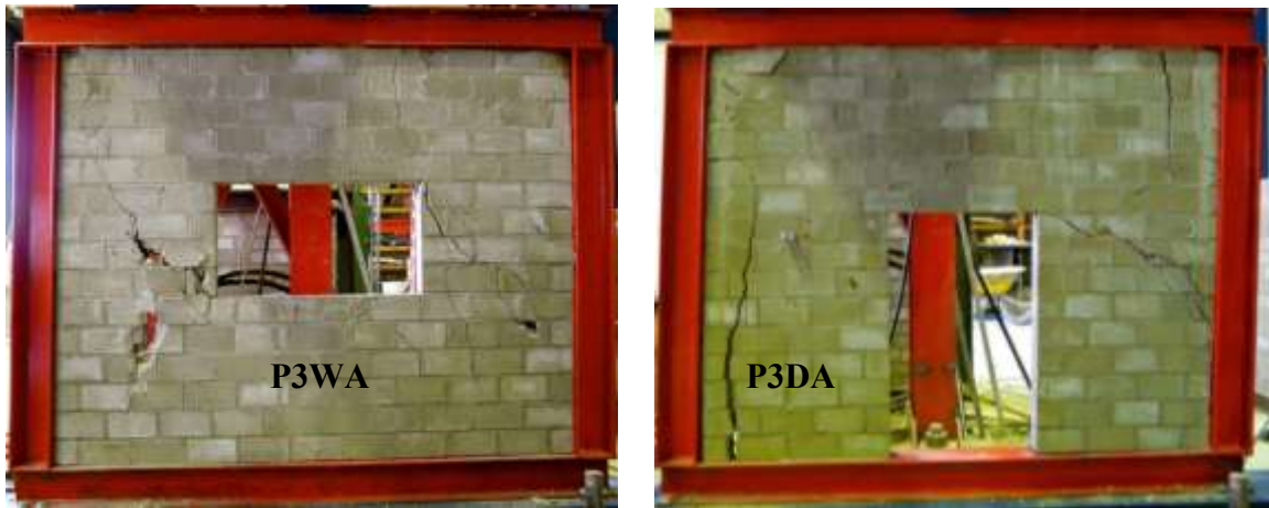
Figure 4.24 Failure of infilled frames with opening.
