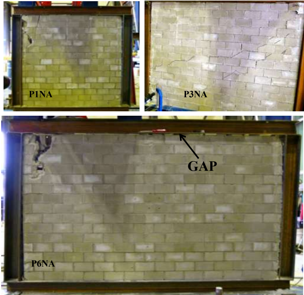
Figure 4.19 Failure of wall specimens
