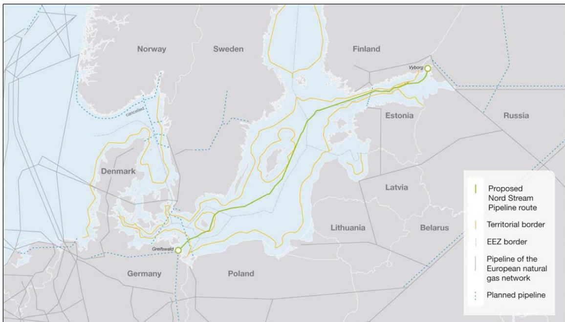
Figure 6.2 Nord Stream Pipeline Route (Source: Nord Stream AG)
