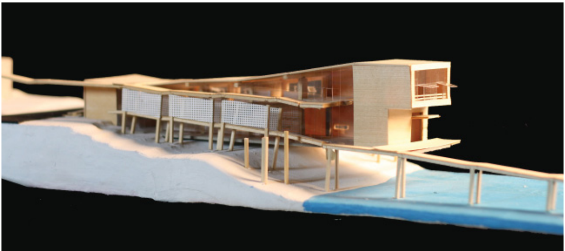
Detail of building model showing boat storage (behind screen) between where the ramps enter the building on the top floor and leave on the main floor.
