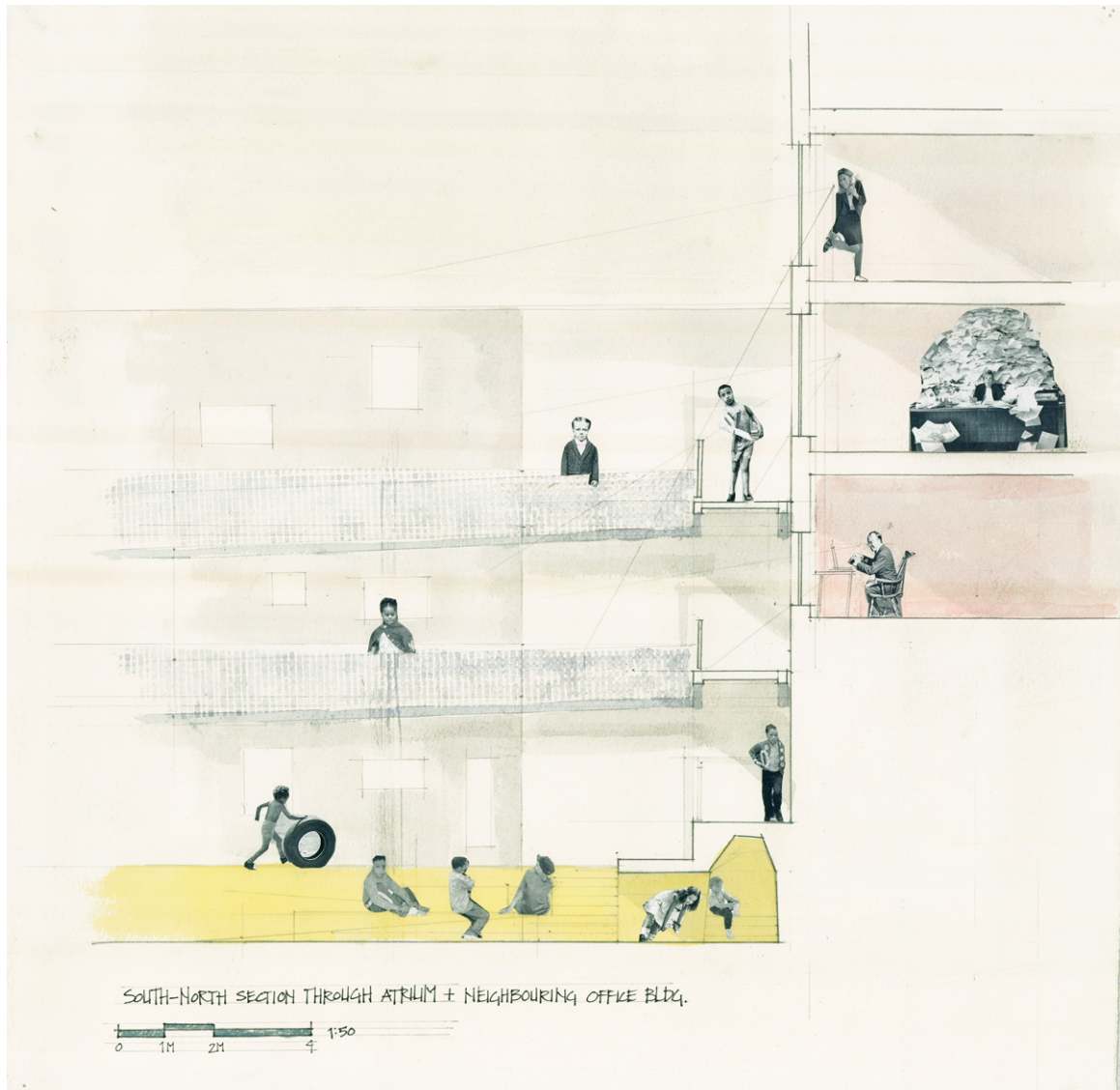
Partial section through the shared openzone, tunnel, atrium, and adjacent office building.
