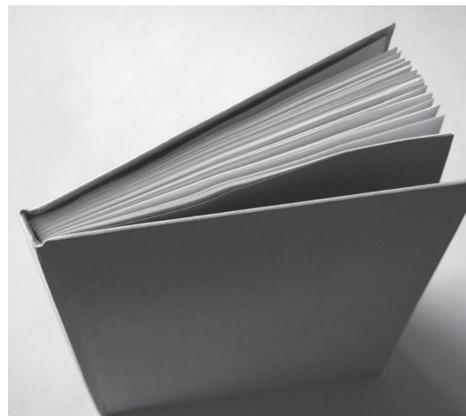
Larger sheets of paper, cut down to 8.5 by 11 inches and folded in half, were used to obtain the correct grain direction
