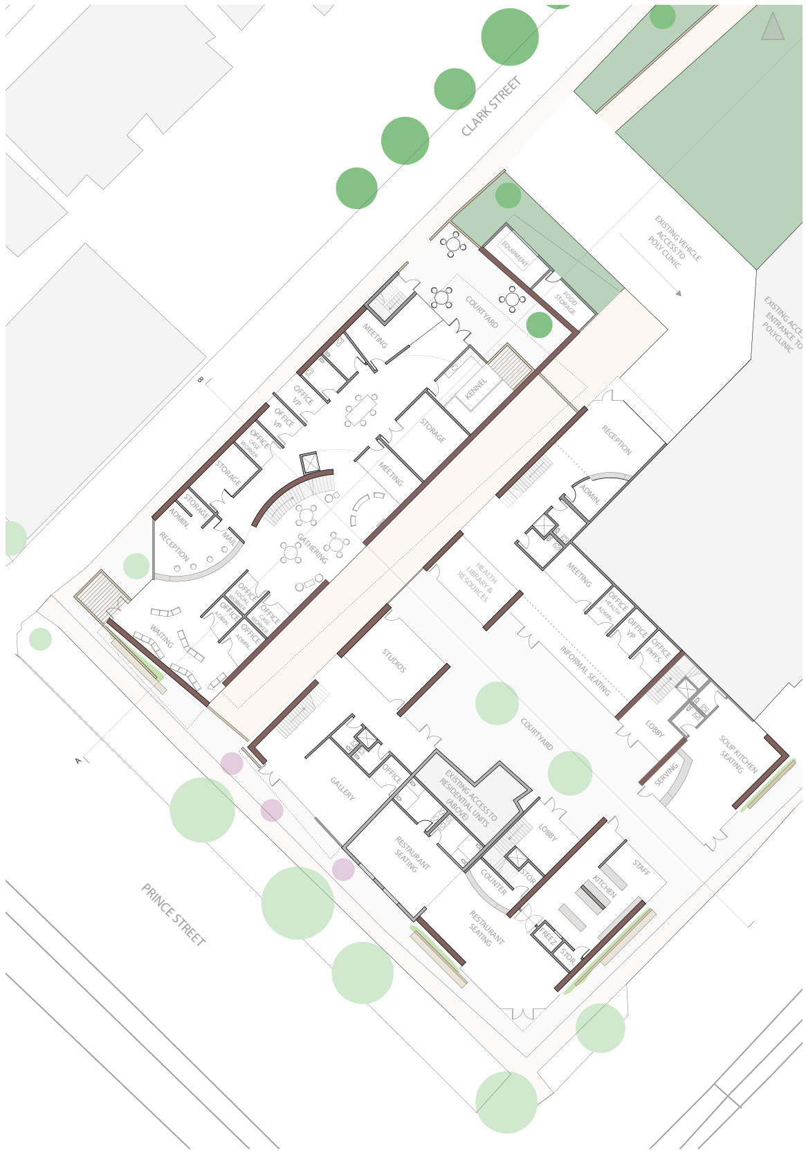
First Floor, Plan, Zoomed In to Show the Shelter, Gallery, Regenerative Health Support Clinic, Soup Kitchen and Restaurant in Relation to the Street, Courtyard, Polyclinic and Existing House.
