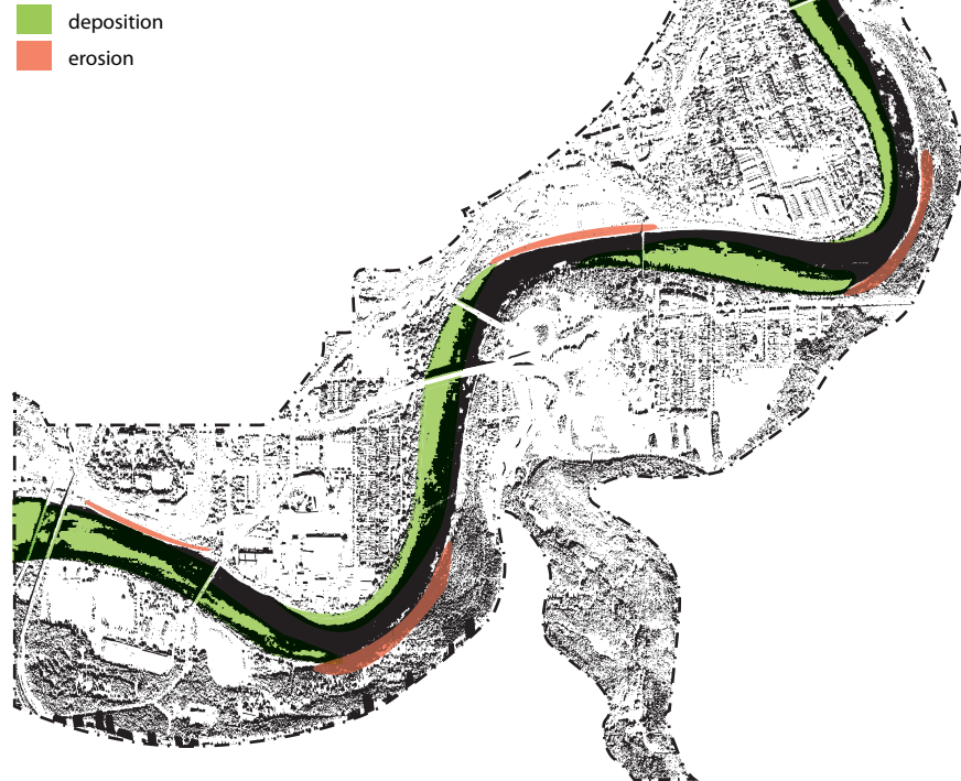
Figure 33. Sediment and Erosion Pattern.
