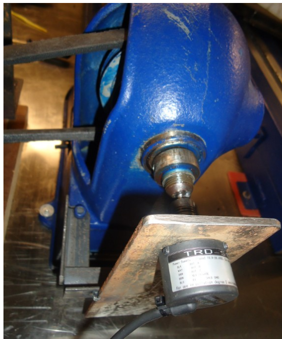
Figure 6.9: Actual setup of the encoder at the head of the lathe.
