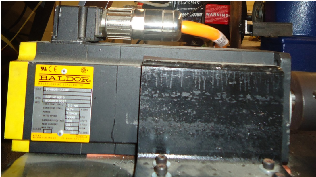
Figure 6.11: Baldor servomotor model BSM80B-233AF
