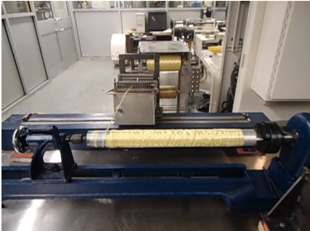
Figure 5.1: Developed prototype filament winding machine
