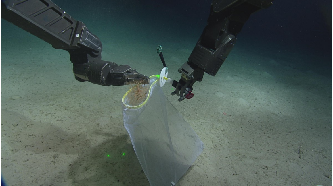
Fig. 2.4 ROPOS manipulator arms placing A. arbuscula colony into mesh collection bag used in 2010. Depth= 1853 m
