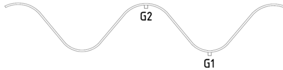
Figure 4-12 – Strain gauge location in structure cross section
