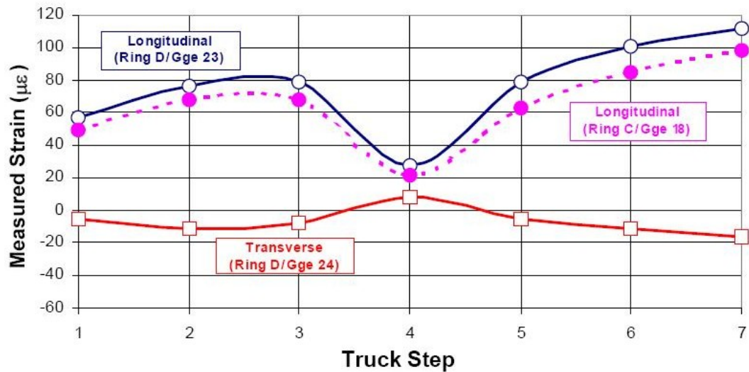
Figure 3-9 – Longitudinal vs. Transverse strains at the crown for non-EC rib (Au & Lam, 2005)
