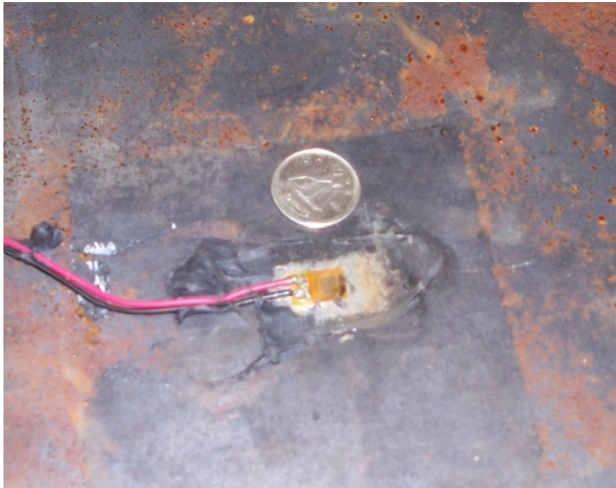
Figure 4-8 – Typical strain gauge
