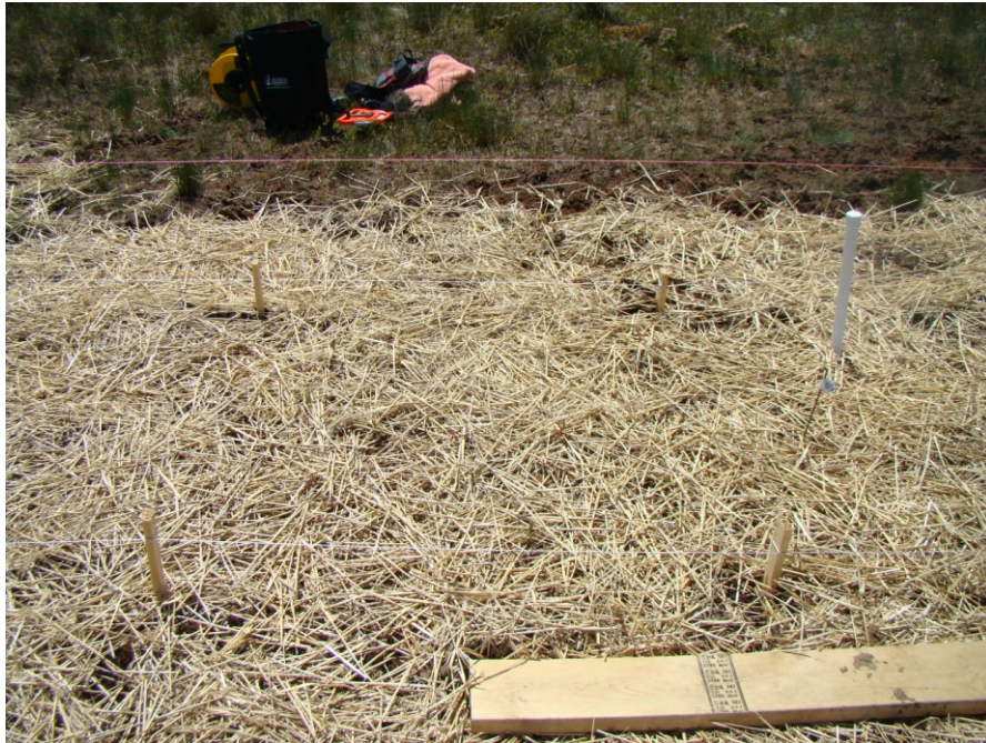
Figure 4.5.1 Example of straw cover with about 85% coverage over treatment. Straw was also applied to the 30 cm buffer zone.
