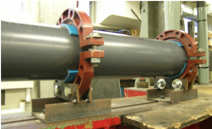
Figure 6-3 Cantilevered boundary condition.
