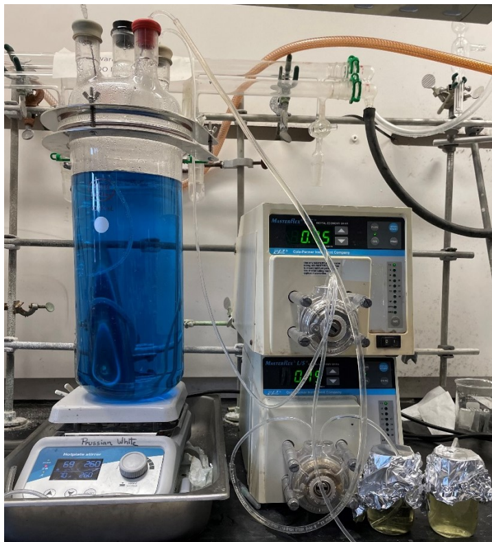
Figure 4.1. Co-precipitation synthesis setup used in this study to produce PBAs.
