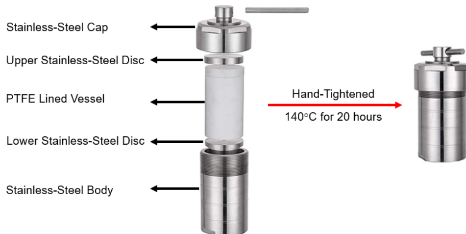
Figure 4.2. Schematic for the hydrothermal reactor assembly used in this study.
