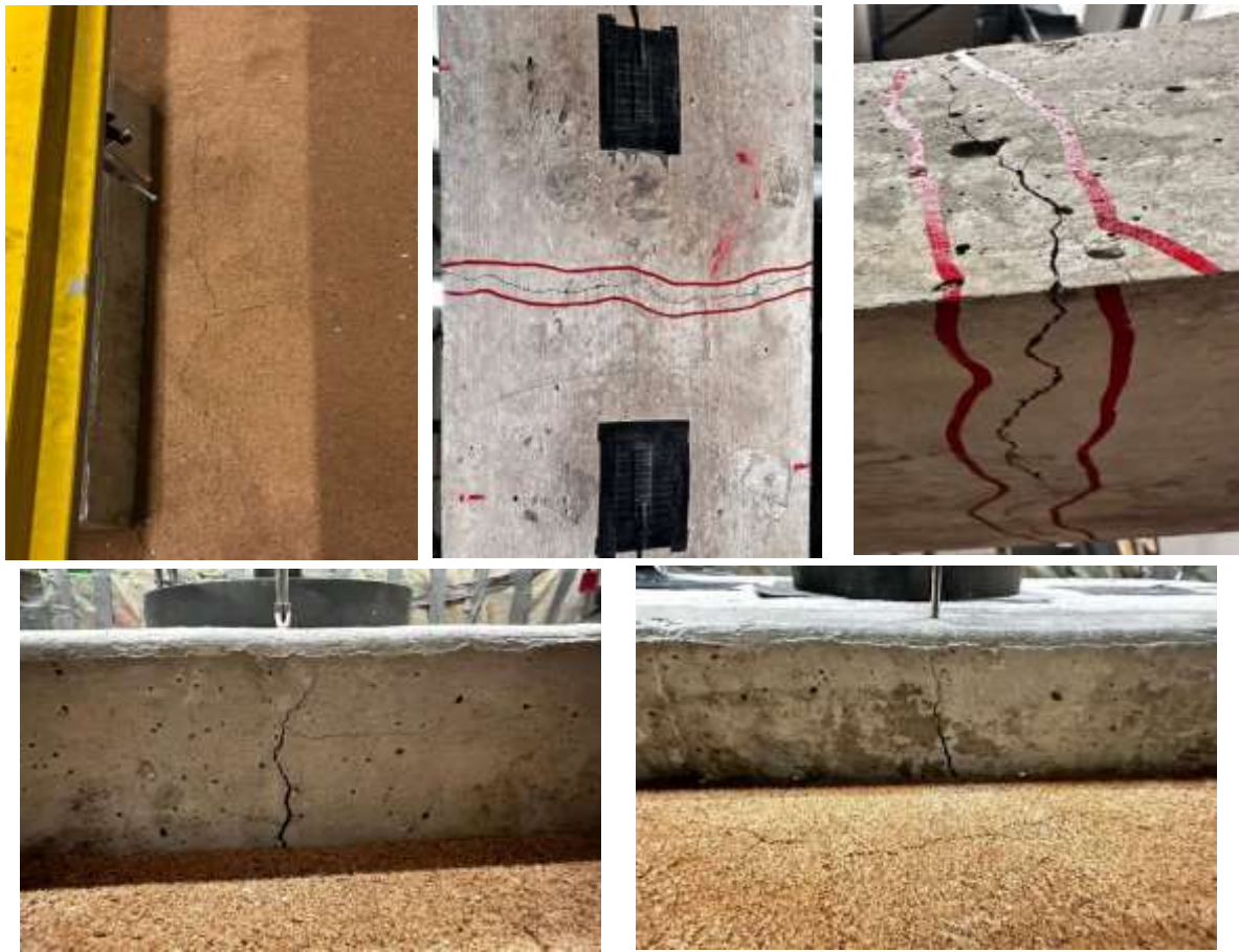
Figure 6.4: (A) Soil Crack at Sections A-A1, B-B1, and Lateral Cracks (B) Flexural Cracks of GFRP-2 Slab
