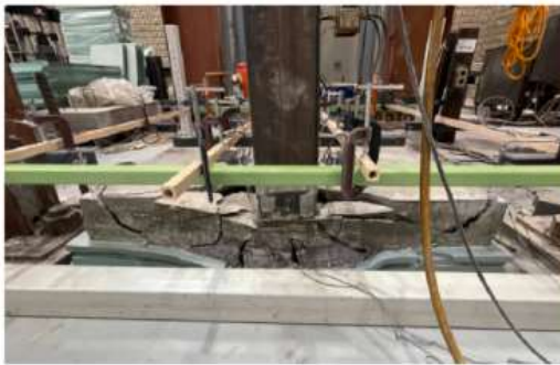
(c) failure in RB-200-EDGE
