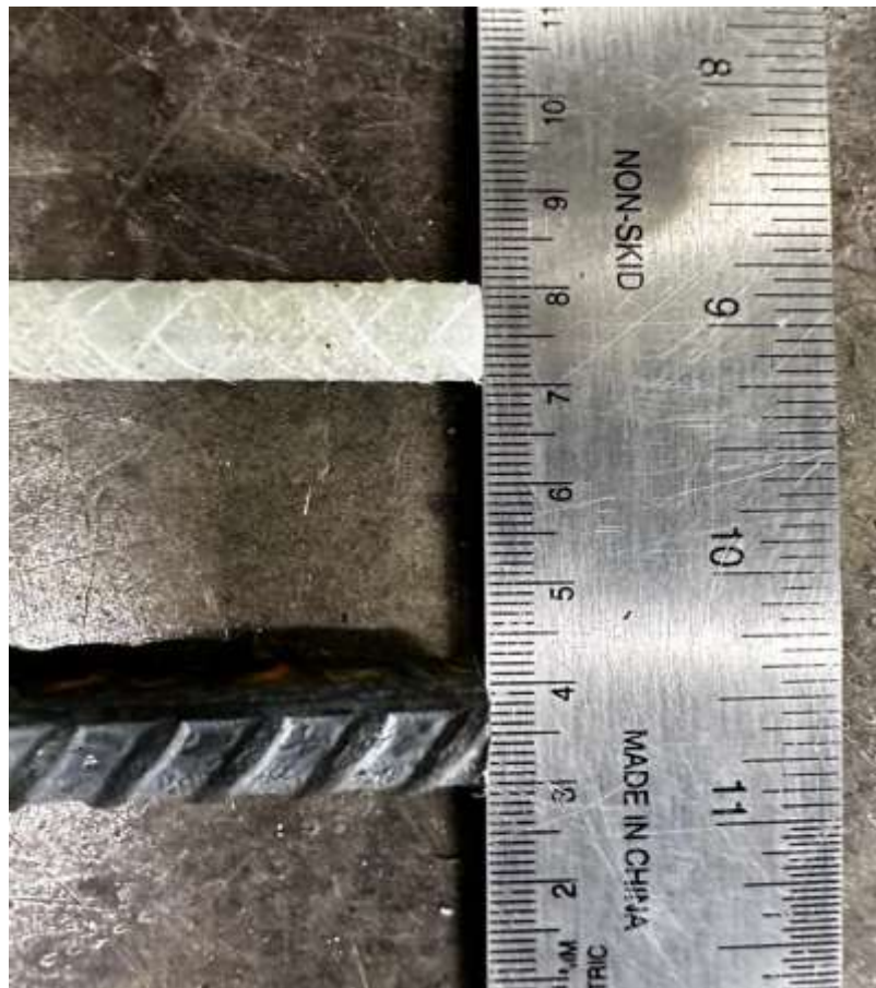
Figure 3.2: V-Rod 46 GFRP Rebar
