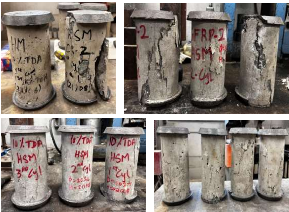
Figure C.2: Cracked Cylinder Specimens
