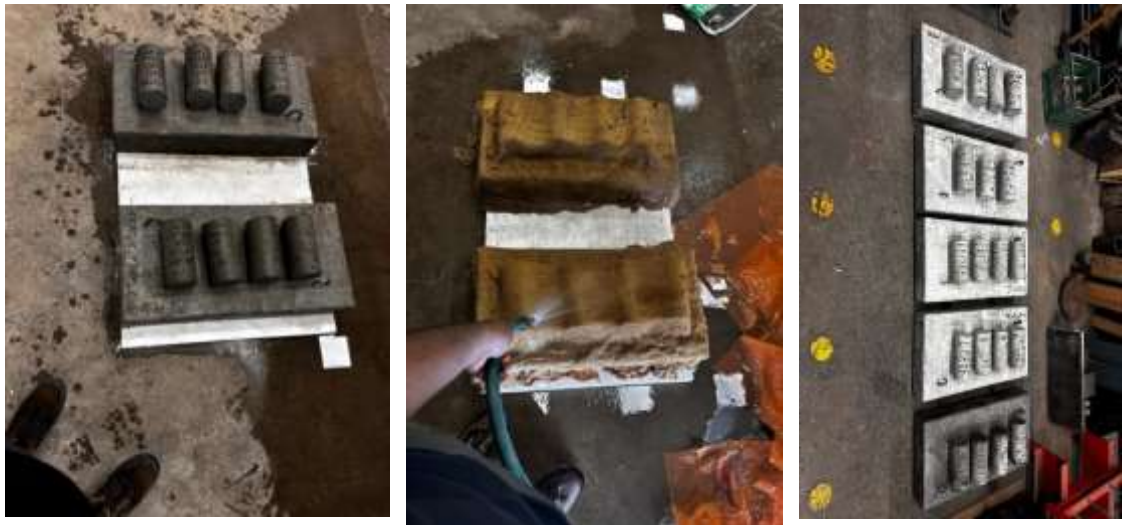
Figure 3.7: Slab Specimen Moist-Curing.
