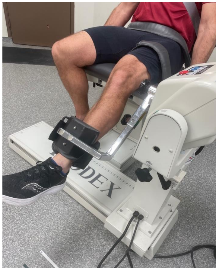
Figure 3-4: Illustration depicting a maximum isometric strength trial for knee flexion and extension.
