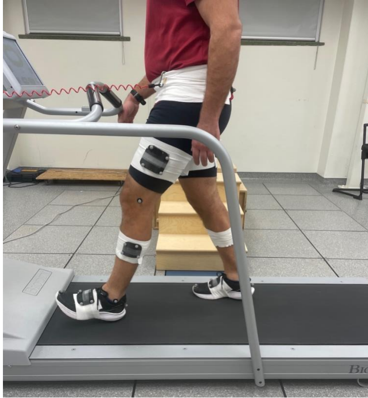
Figure 3-3: A sagittal view of the lower extremity portion of the marker set during the treadmill walking protocol.
