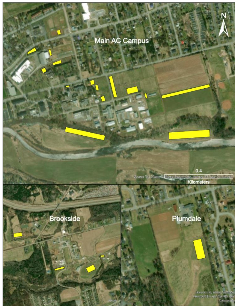
Figure 3 Twenty locations with potential for implementation of agrivoltaic farming on the Dalhousie Campus in Truro, Nova Scotia, Canada. Locations were identified by both our research team and by university staff through focus groups. The PV system size is identified by yellow rectangles, where smaller rectangles generate less energy than larger rectangles. The polygons and titles were created by A. Hebert. The basemap was created by ESRI with a NAD 83 spatial reference. The map was created on March 26 th , 2024.
