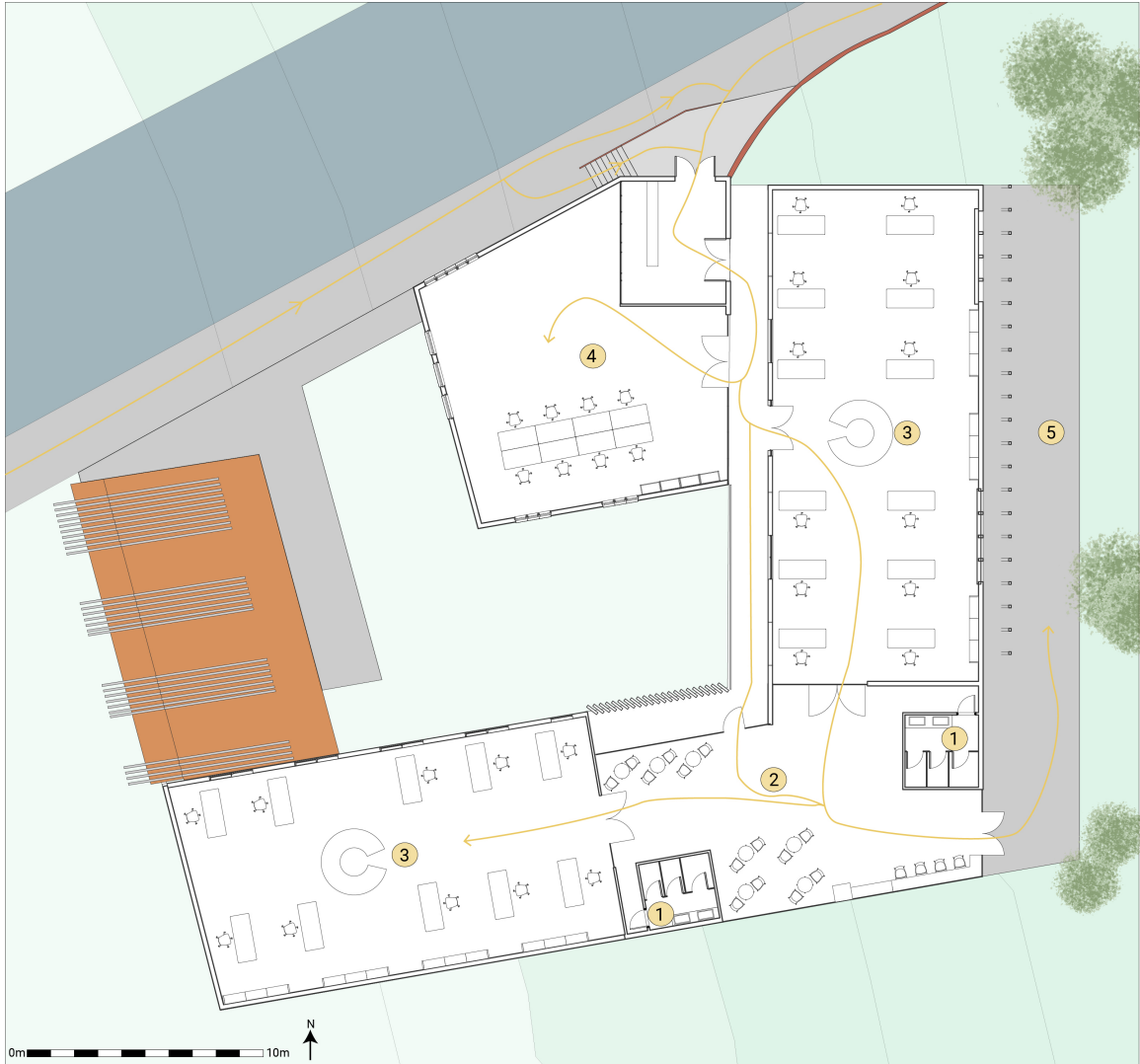
Figure 37: Costume Design Trade School Level 1 floor plan. The yellow arrows show circulation paths throughout the site.
