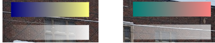
Figure 6.6: LEFT: Ukraine, the default colourmap on the top. Ukraine with its luminance converted to alpha at the bottom. RIGHT: Saga, the colourmap used in the study on the top. Saga with its luminance converted to alpha at the bottom. Saga is more isoluminant than Ukraine.
