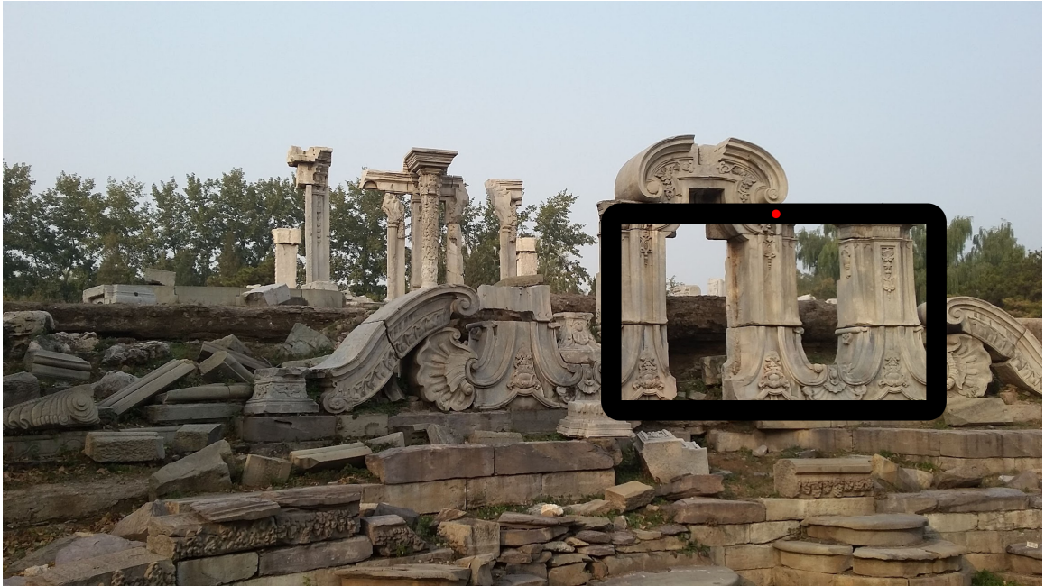
Figure 2.6: While a display screen may have the same lightness with the environment, the actual luminance can be much higher. The OST-HWD may have difficulty mounting on such area.
