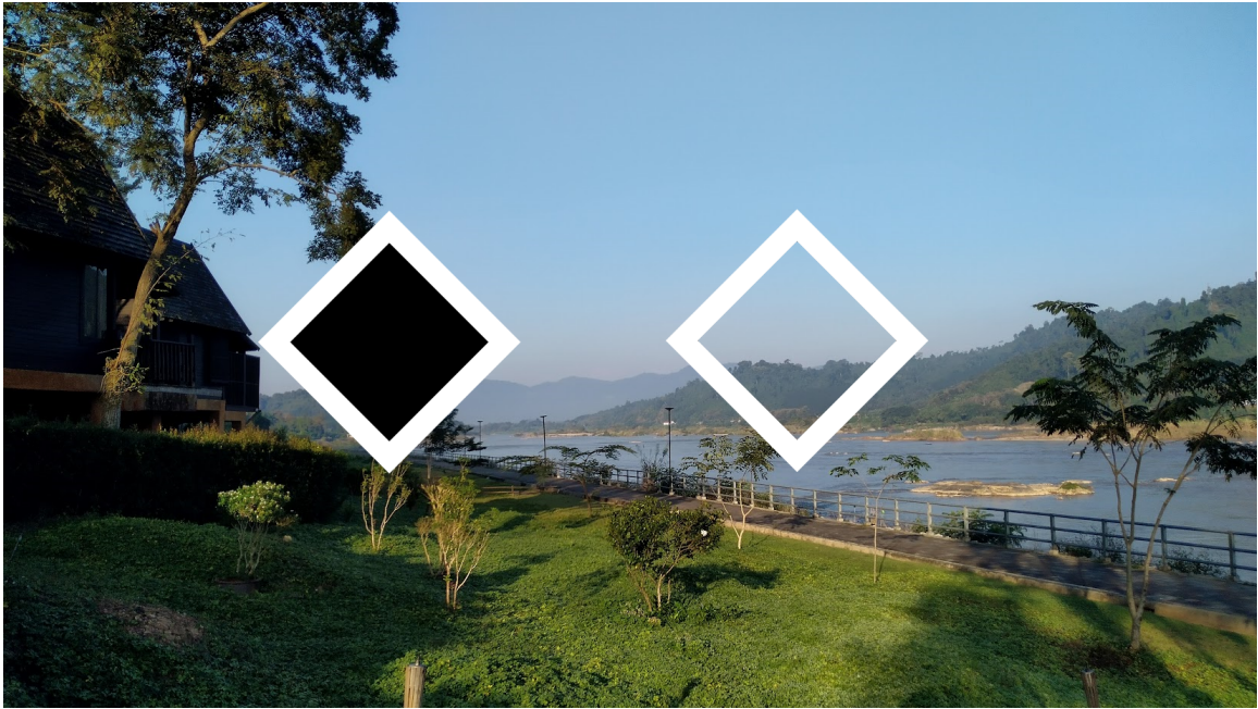
Figure 2.5: The left diamond represents a black diamond shape with a white outline displayed that one may expect. The right diamond shows how OST-HWDs render it; the black fill is completely transparent.
