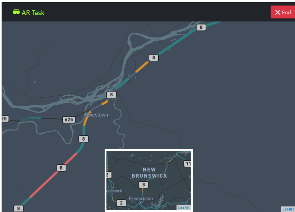
Figure 5.2: The tablet interface. The smaller inset is the virtual touchpad, which allows for rapid scrolling of the entire area. Tapping “End” means all sub-tasks have been completed.
