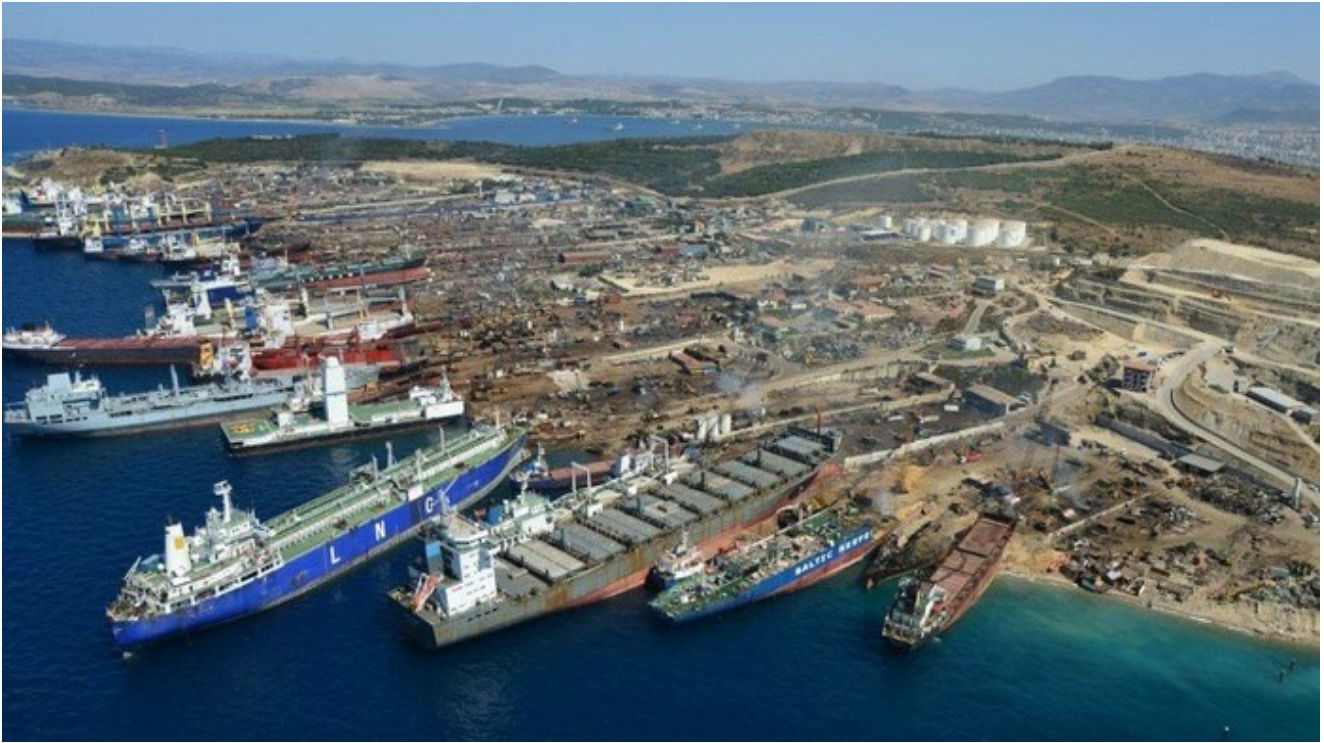
Figure 14. EoL Ships Beached at a Turkish Recycling Yard on a Slipway Source: https://shipbreakingplatform.org/our-work/the-problem/Türkiye/ © Ship Recyclers' Association of Türkiye
