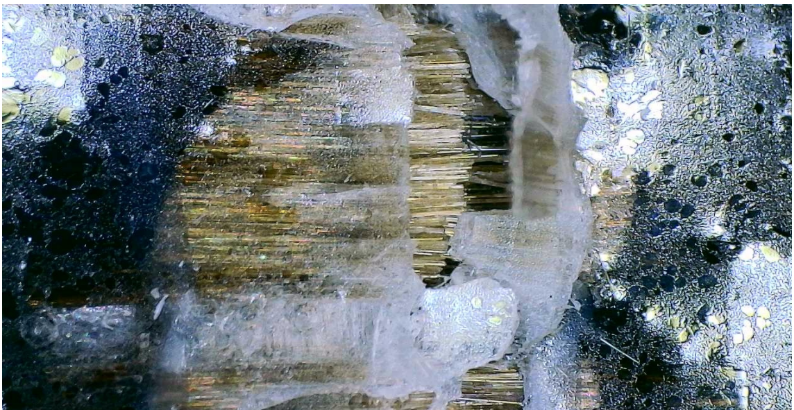
Figure 6-29: Digital microscope images of the failure region of basalt Elium compression Sp 5 (side and top views, respectively)
