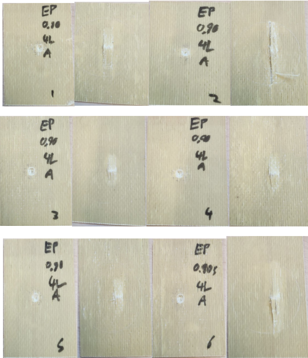
Figure 6-40: Post HVI view of Kevlar-29 HVI specimens (front and rear, respectively)
