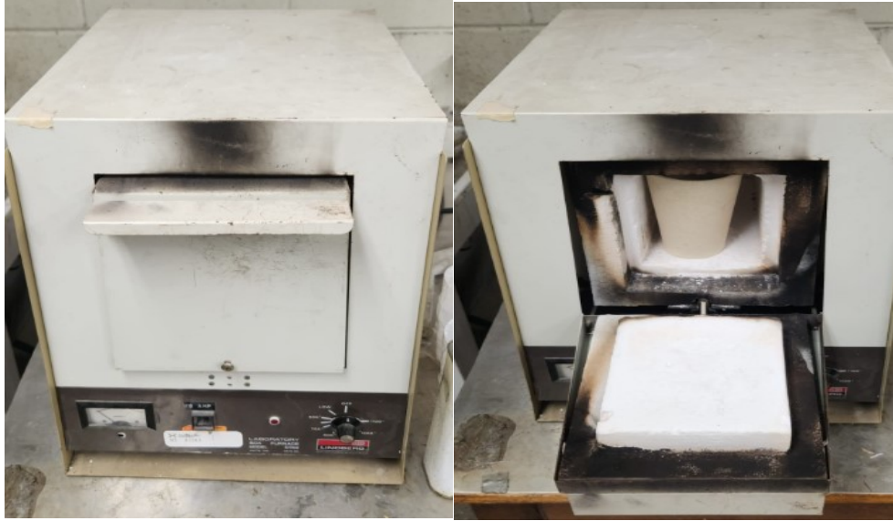
Figure 5-2: Furnace used in resin burn-off test
