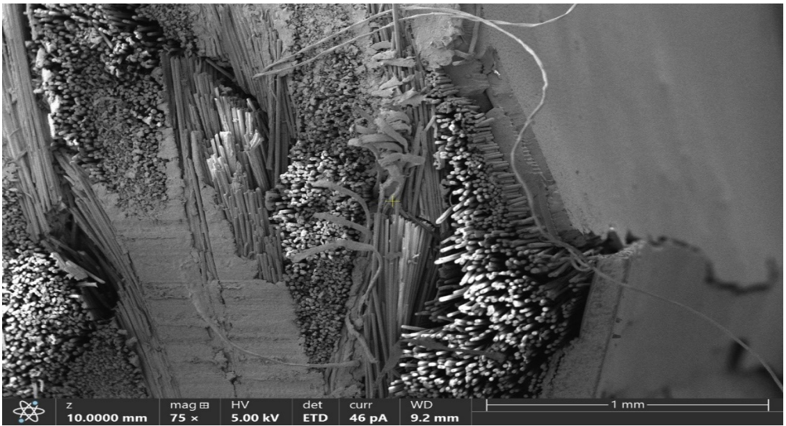
Figure 6-31: SEM images of the failure region of basalt epoxy compression Sp 3
