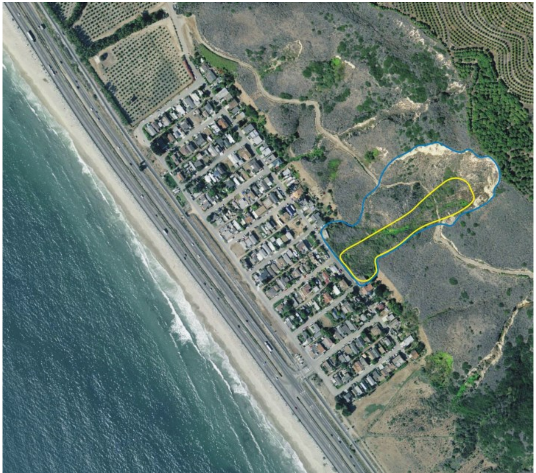
Figure 6 Aerial photograph of the landslide which occurred in 1995 outlined in blue color and subsequent remobilized area which occurred in 2005 outlined in yellow color [84].
