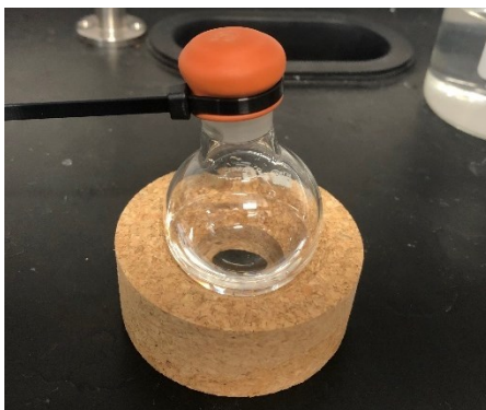
Figure 13: Representative pre-polymerization solution in a 50 mL round bottom flask; sealed with an orange septum and black zip tie
