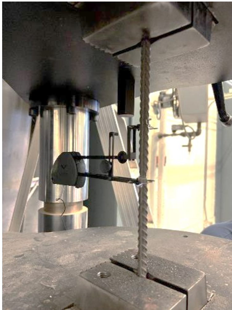
Figure 7.11. Reinforcement steel rebar specimen typical testing configuration.
