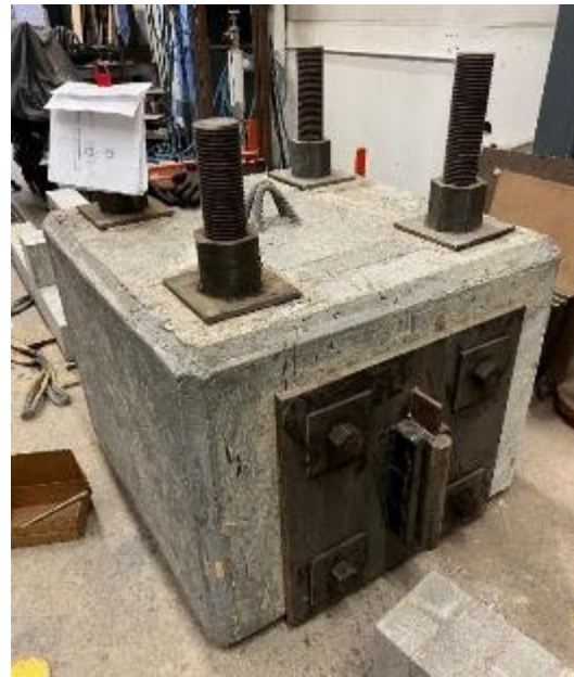
(c) Rigid cubic concrete support.
