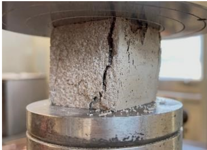
Figure 7.5. Mortar specimen typical failure.
