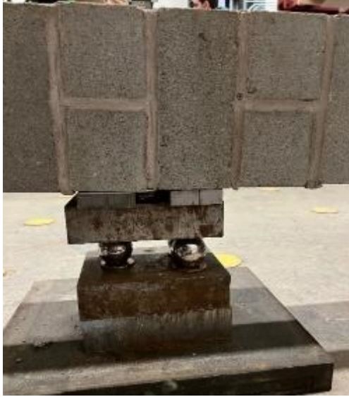
Figure 3.10. Steel balls for weight elimination.
