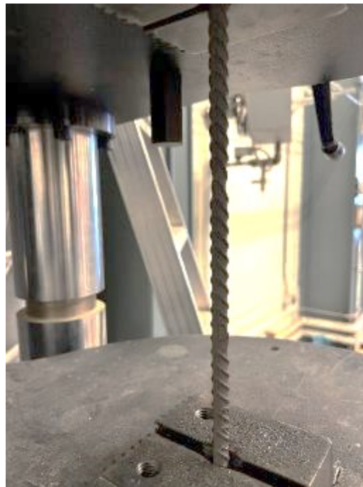
Figure 7.12. Typical reinforcement steel rebar specimen failure
