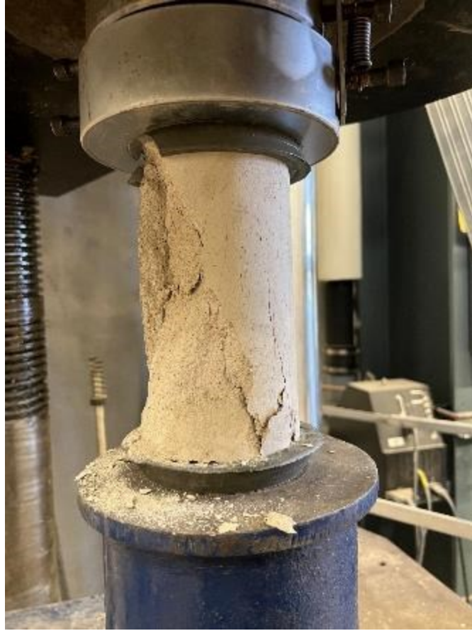
Figure A.7. A typical failure of grout specimens.
