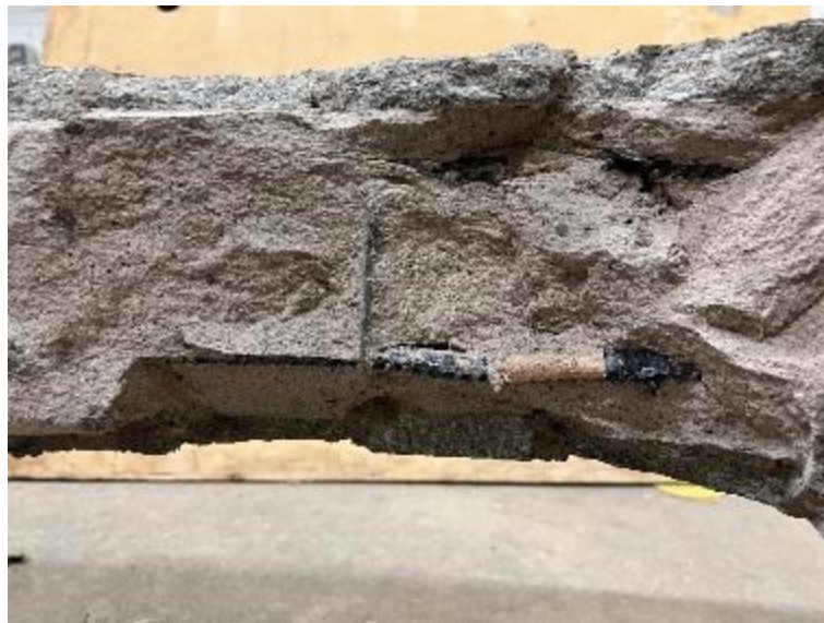
Figure 4.7. Reinforcement local buckling in specimen MC.
