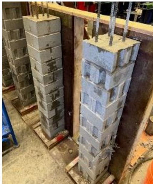
(c) After grouting
