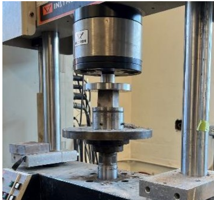
Figure 7.4. A typical testing configuration of mortar specimens.
