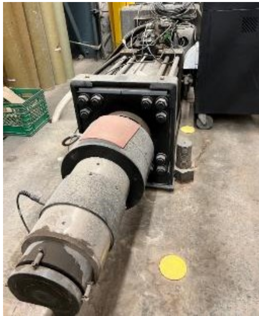
(b) 2 MN actuator and its rigid support.
