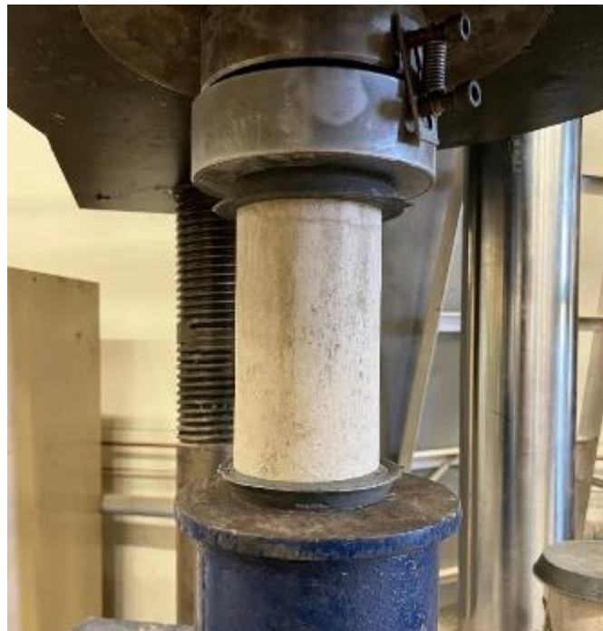
Figure 7.6. Grout specimen typical testing configuration.
