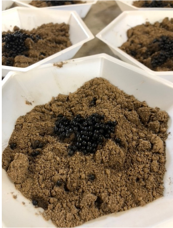
Figure 21. Mixing Pb 2+ spiked BAC with soil before putting into mason jars for microbial respiration experiment.
