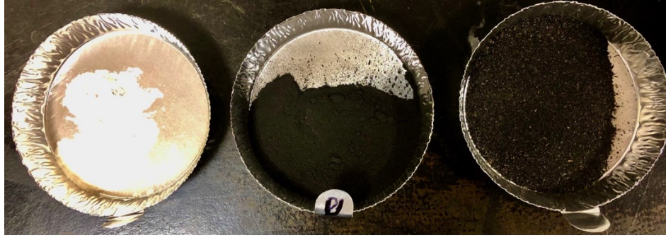
Figure 2. 4 % (w/v) of biochar and 1 % (w/v) of alginate weighed prior to adding to deionized water and mixing on the magnetic stirrer.
