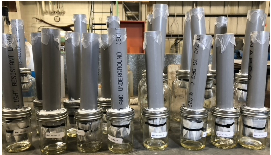
Figure 20. Leaching Experimental Setup. BAC-10 treatment section at day 3 with a total of 18 experimental units.
