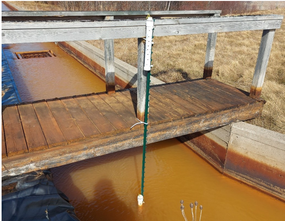
Figure A.10 HOBO pressure transducers with high flow in channel between settling pond and constructed wetland for System 1.
