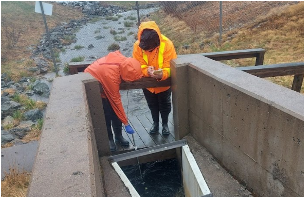
Figure 4.6 Velocity measurement using flow meter at wetland outlet of System 1 on April 26 th , 2021.
