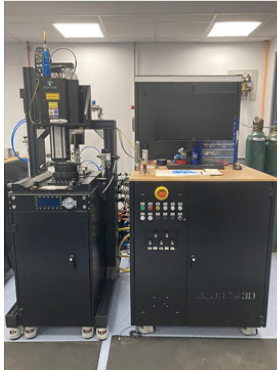
Figure 23: Aconity 3D LPBF machine utilized for all builds.
