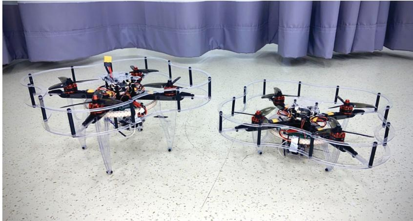
Figure 1.1: COEX Clover 4.2 drones at the Advanced Control and Mechatronics Lab, Dalhousie University.
