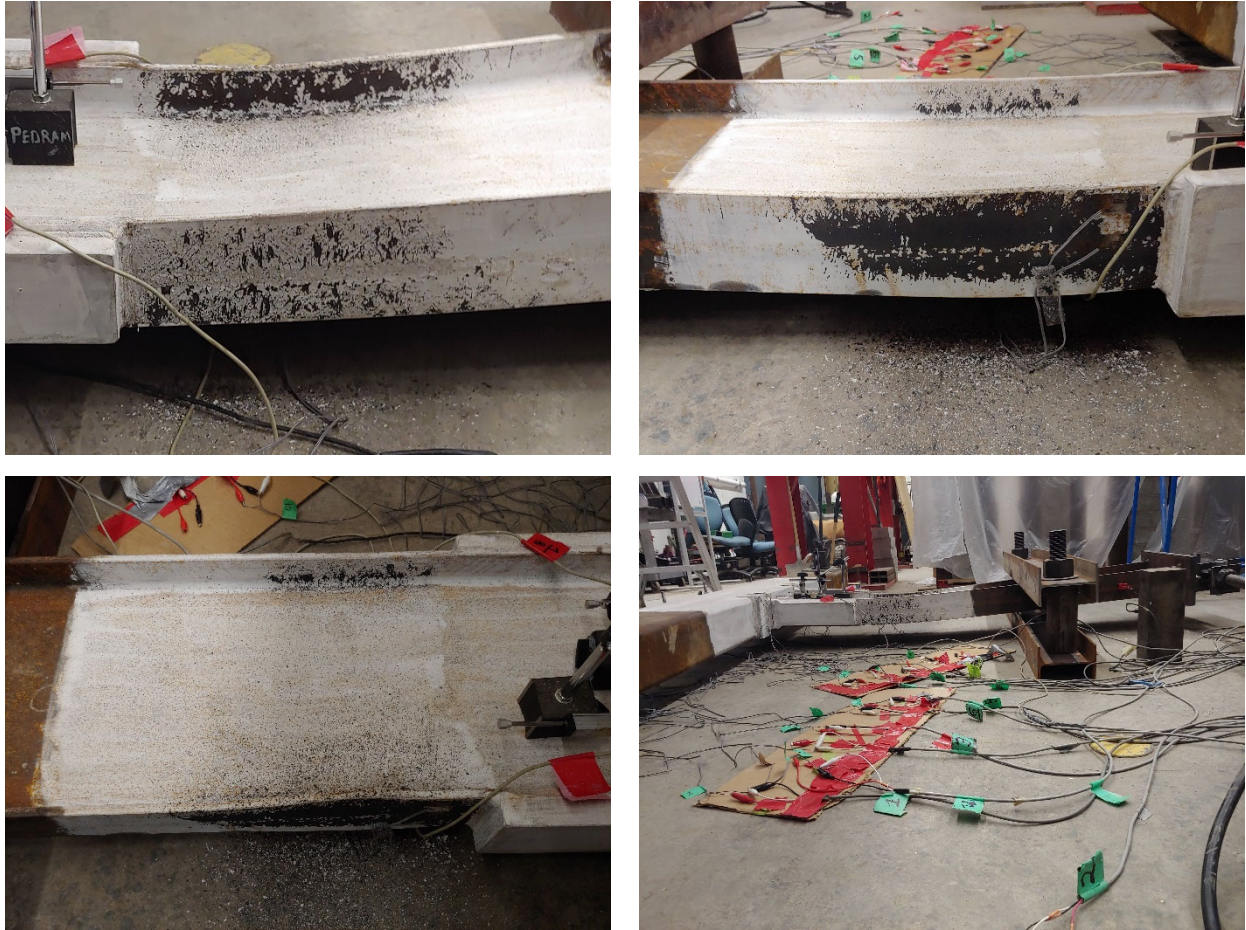
Fig. H.8. Doubler Plate post-testing photos
