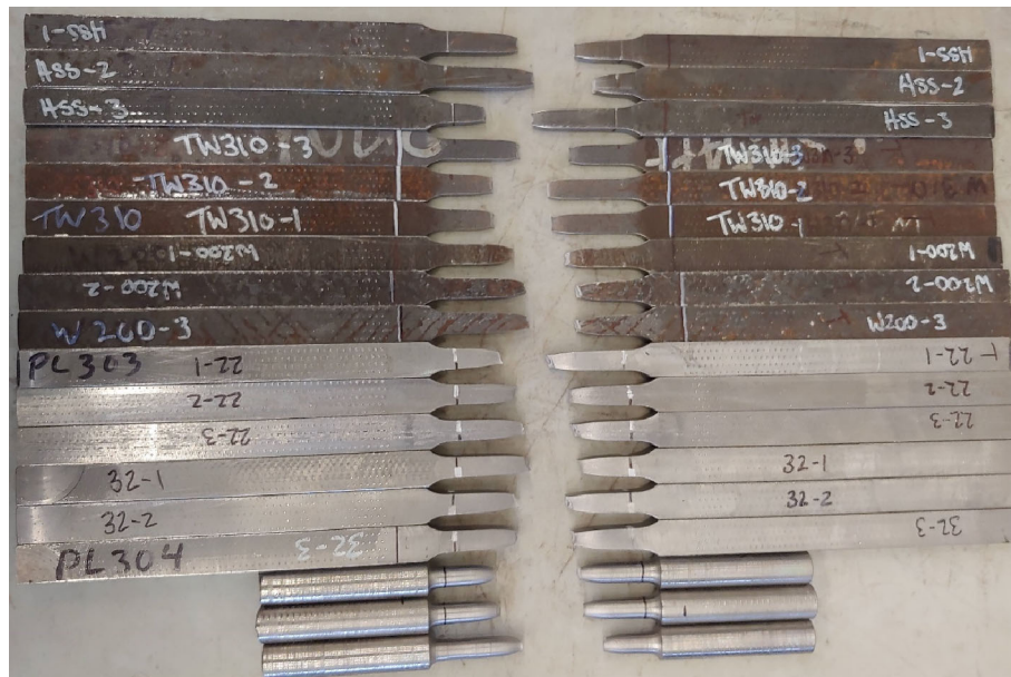
Fig. 4.2. TC post-fracture for base metals and all weld metal
