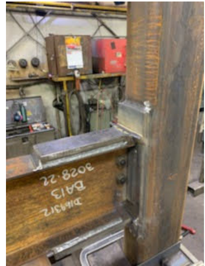
(f) fully welded connection
