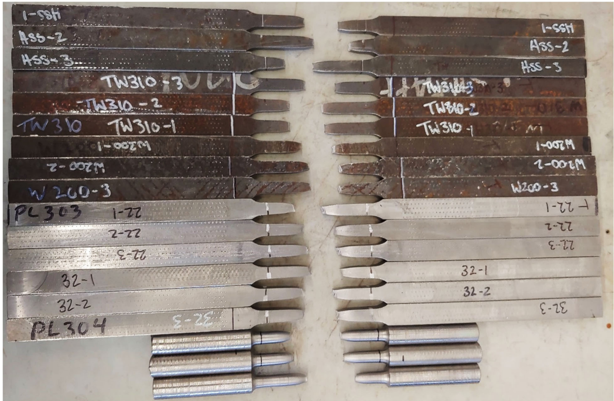
Fig. G.1. Tensile coupons (post-testing)
