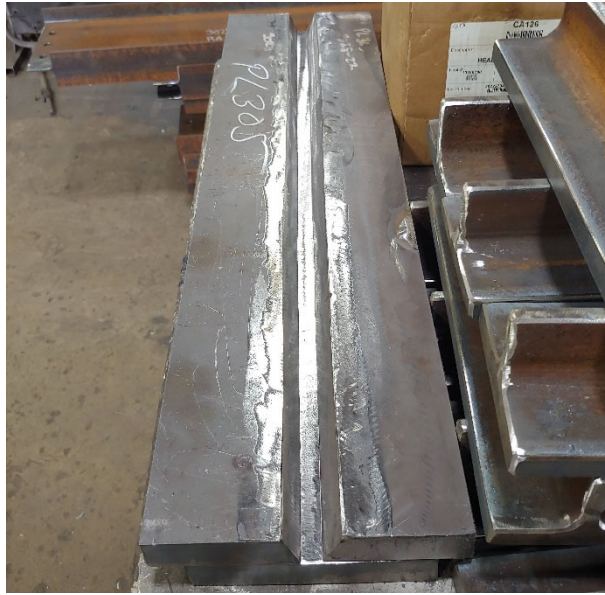
Fig. 4.9. All weld metal groove assembly plates fabricated before weld metal added
