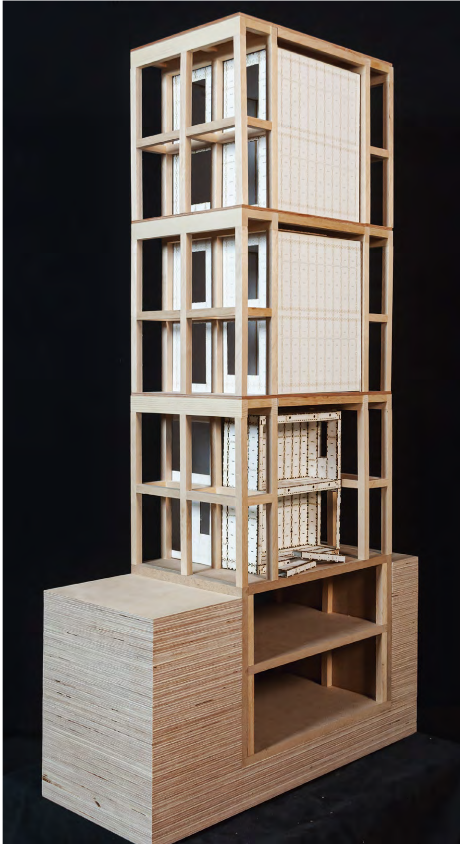
The Key Section Model Part B: Base Building with WikiHouse Components of Infill (Note the facade is not shown in these representations).
