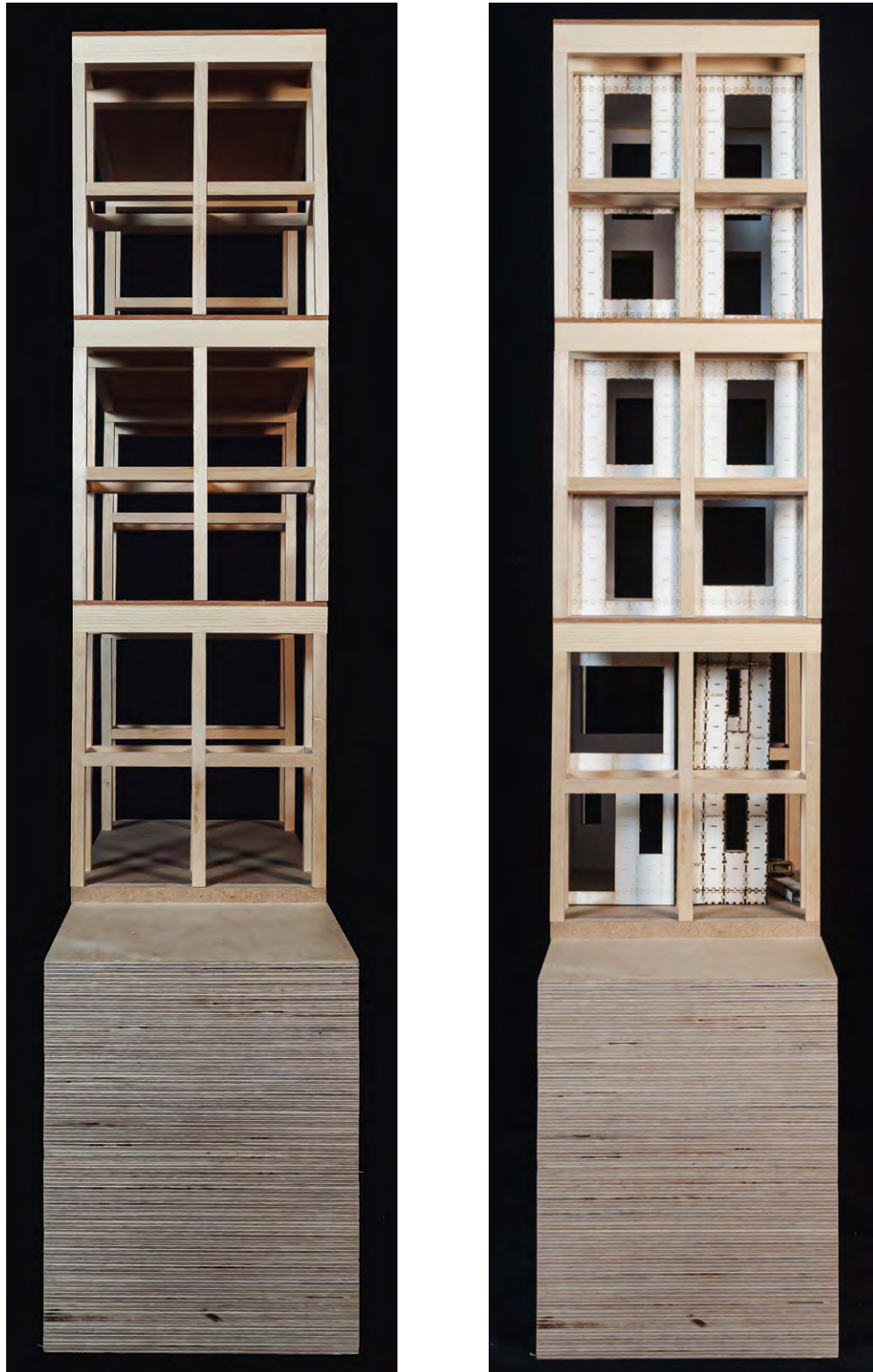
The Key Section Model Part A: Base Building, Part B: Base Building with WikiHouse Components of Infill (Note the facade is not shown in these representations).
