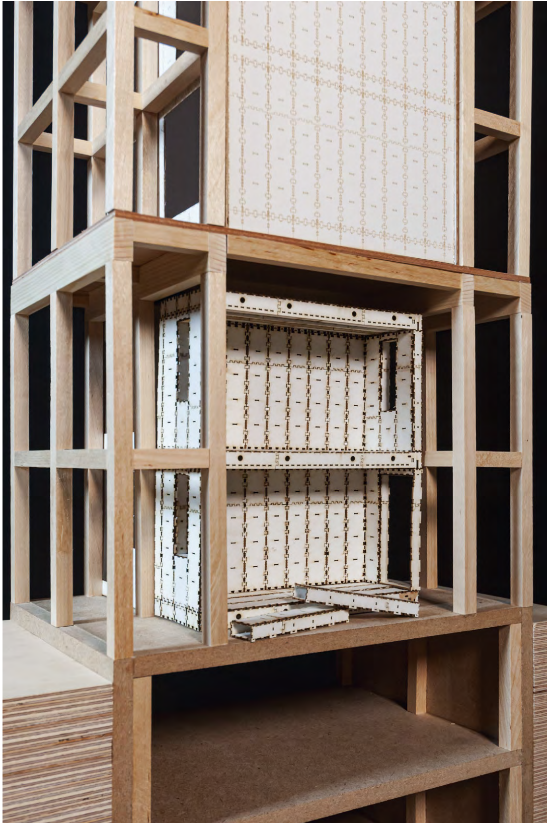
The Key Section Model Detail Shot Part B: Base Building with WikiHouse Components of Infill (Note the facade is not shown in these representations).
