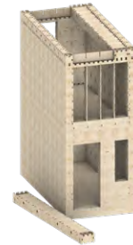
Place Floor Components on Combs
