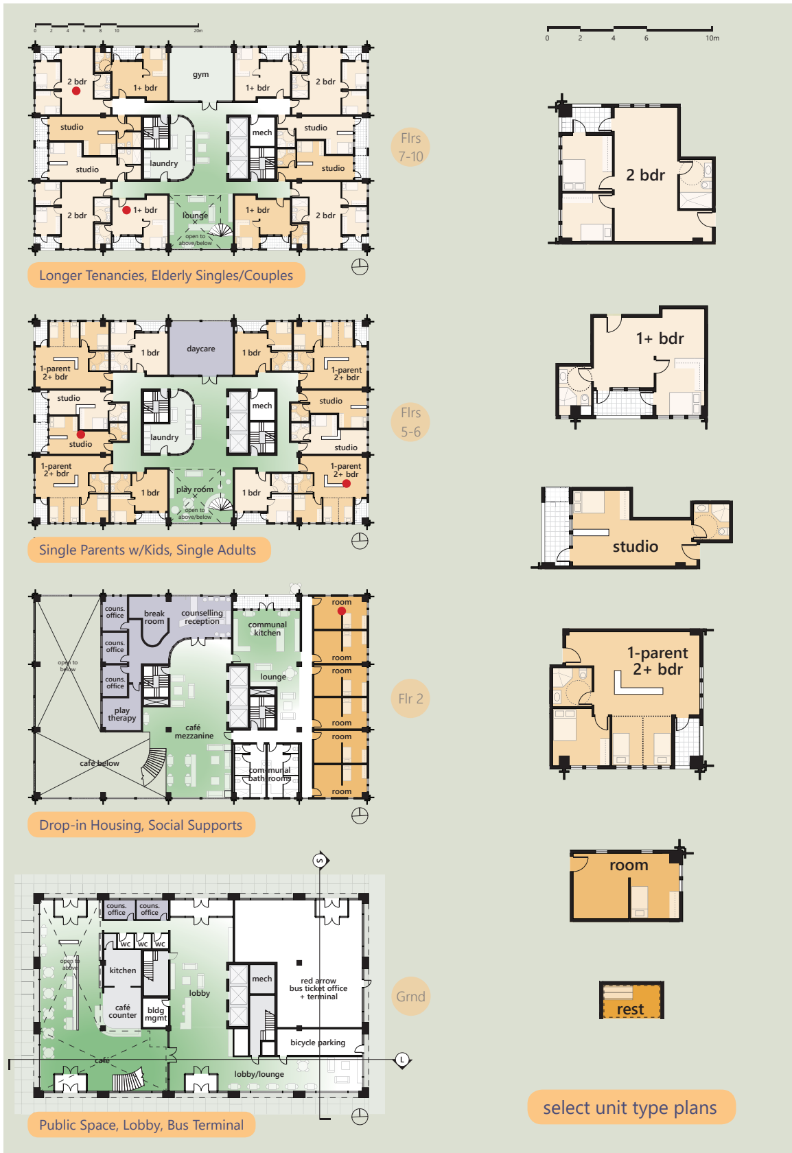
Typical 3SP Tower floor plans, with select examples of residential unit types emphasized
