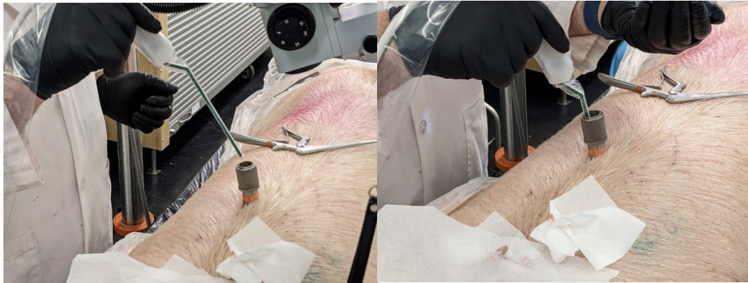
Figure 4.7 Ex vivo porcine spine imaging with an inserted steel tube where a) the probe is held above to compare the probe tip to the entrance of the tube and b) the probe has been lowered into the tube.
