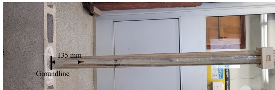
Figure 5-19 The strain gauges' locations along the 3D poles.
