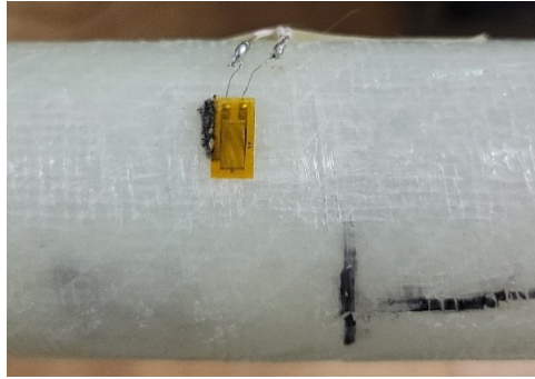
Figure 6-4 The strain gauge mounted for measuring the hoop strain.
