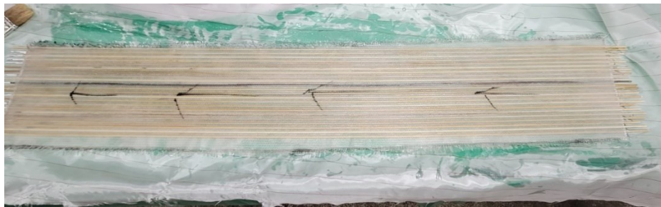
Figure 5-13 Fabrication of the WCGFRP before rolling on the mandrel.
