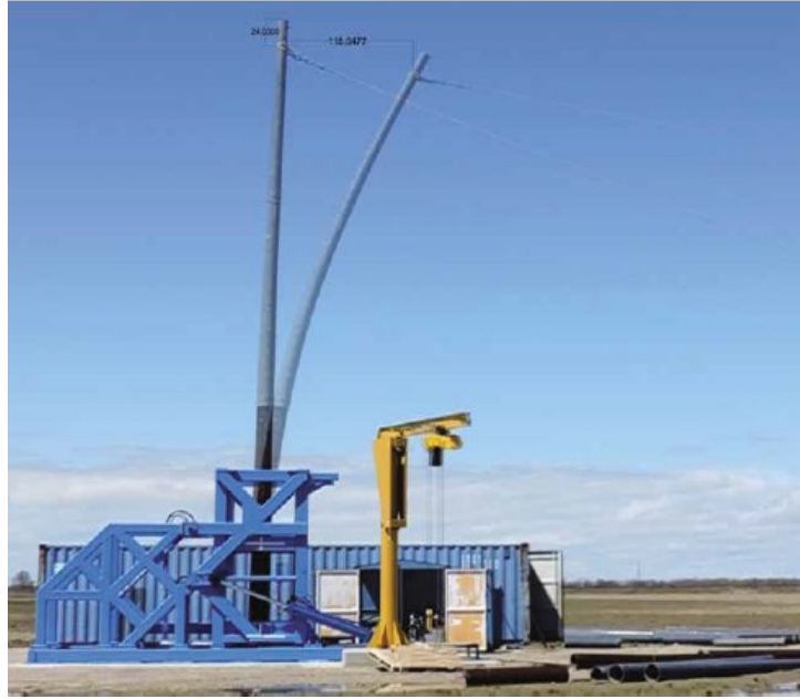
Figure 1-7 Illustration of the full-scale flexural test of an FRP pole based on the ASTM D1036-99 (ASCE, 2019).
