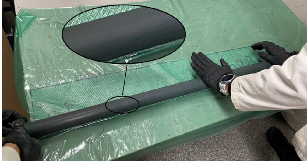
Figure 5-11 Prepreg was rolled up to the surface-prepared mandrel.
