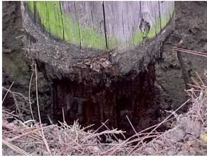
Figure 1-2 A wood pole rotted below the groundline due to the fungi attack (Jackson, 2012).
