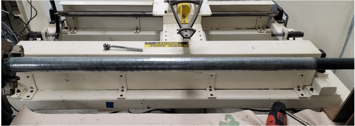
Figure 5-12 A top module wrapped with shrink tape.
