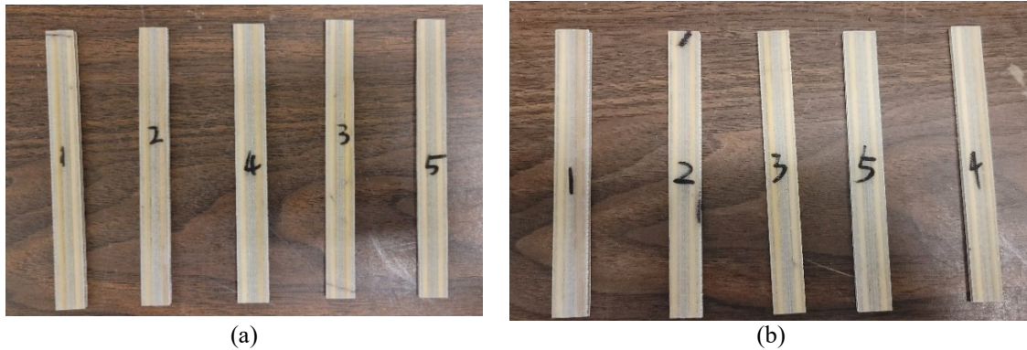
Figure 3-3 Prepared specimens for (a) flexural test and (b) compressive test.
