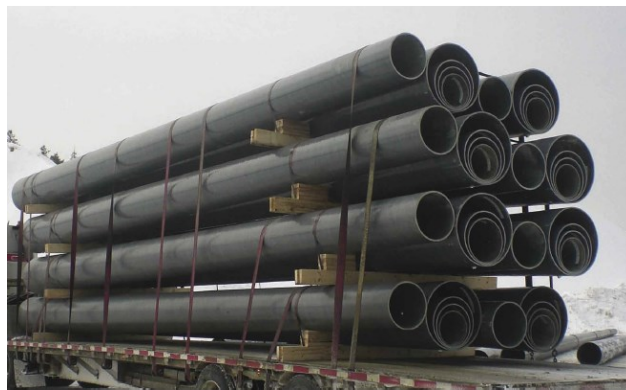
Figure 1-3 Transportation of the nested 38.1m modular poles (ASCE, 2019).
