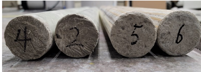
Figure 5-17 Cross-sectional view of the partially concrete-filled poles.
