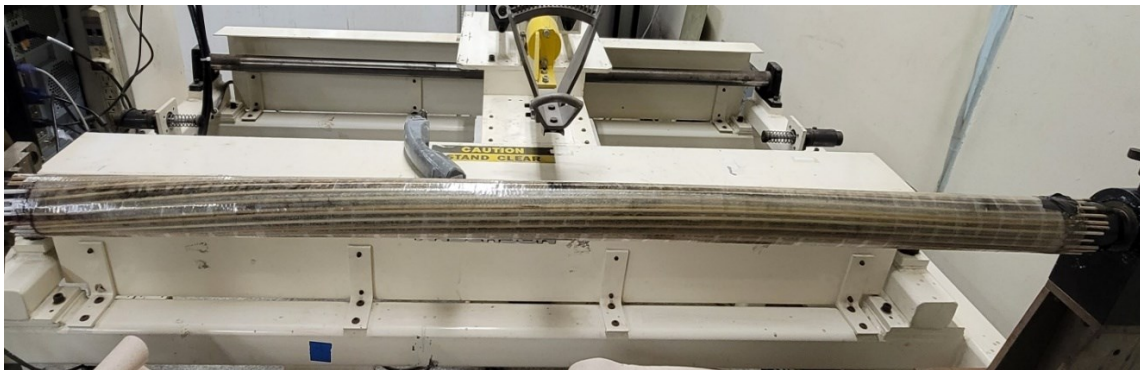
Figure 5-14 A 3D pole wrapped with shrink tap after heating.
