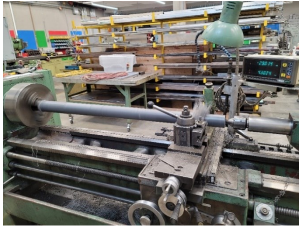
Figure 5-2 PVC rod being turned on Lathe.
