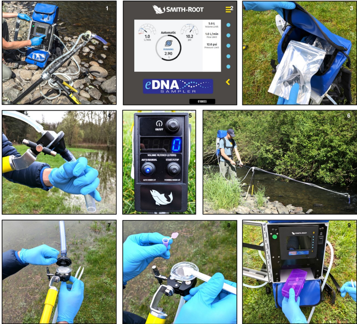
Figure 2.1: Smith Root eDNA sampler performing sample capture and filter storage immediately after capture. Reprint from [15].
